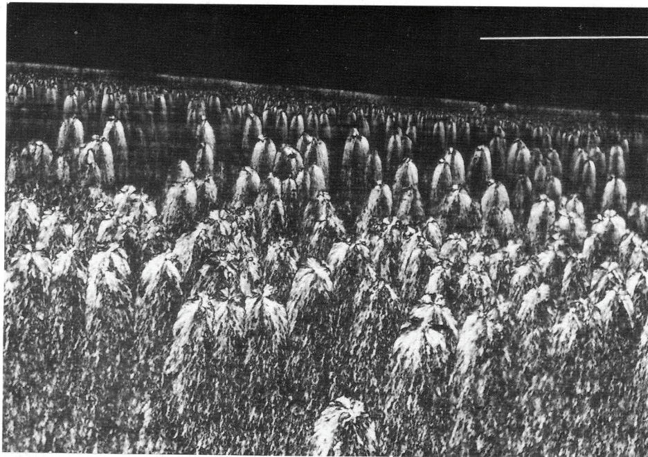
Figure 2-27: Section of acetal; crossed polars. Bar = 100 \mu\text{m} [63].
