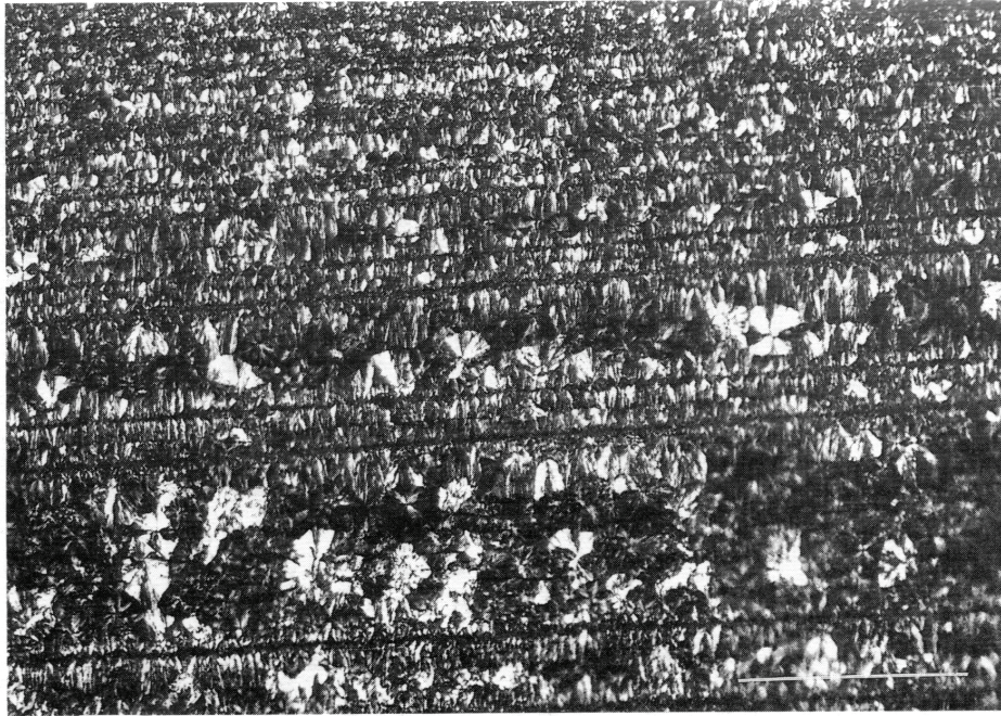
Figure 2-25: Section of polypropylene; crossed polars. Bar = 100 \mu\text{m} [63].
