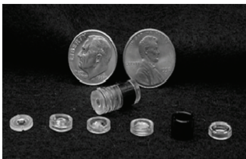
Fig. 3. Injection-molded plastic objective lens assembled and disassembled with U.S. coins.
