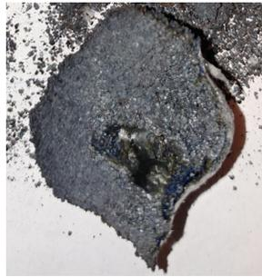
**Figure 33:** Melting within the bed in one of the tests of the second campaign
