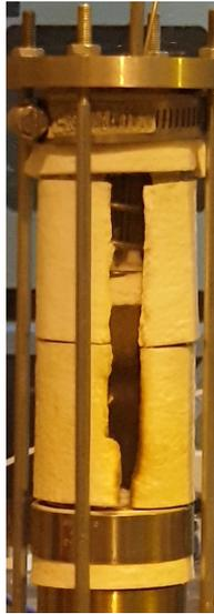
**Figure 34:** Placing ceramic wool as thermal insulation around the quartz tube to reduce the heat loss to the environment
