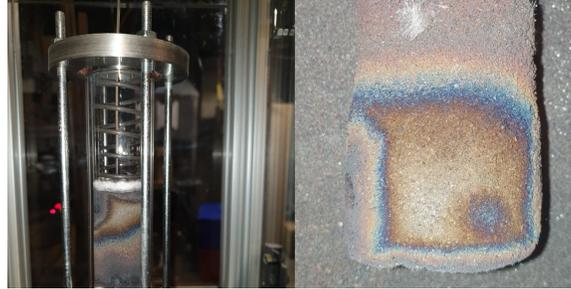
**Figure 30:** Colourful iron hydroxides ( $\text{Fe}(\text{OH})_2$  and  $\text{Fe}(\text{OH})_3$ ) produced during the preheating process.
