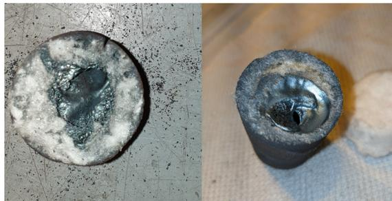
**Figure 29:** An oxidized iron bed produced in the first campaign
