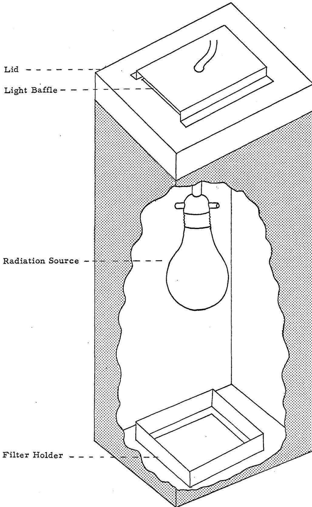
Black aluminium box used to filter visible light.
