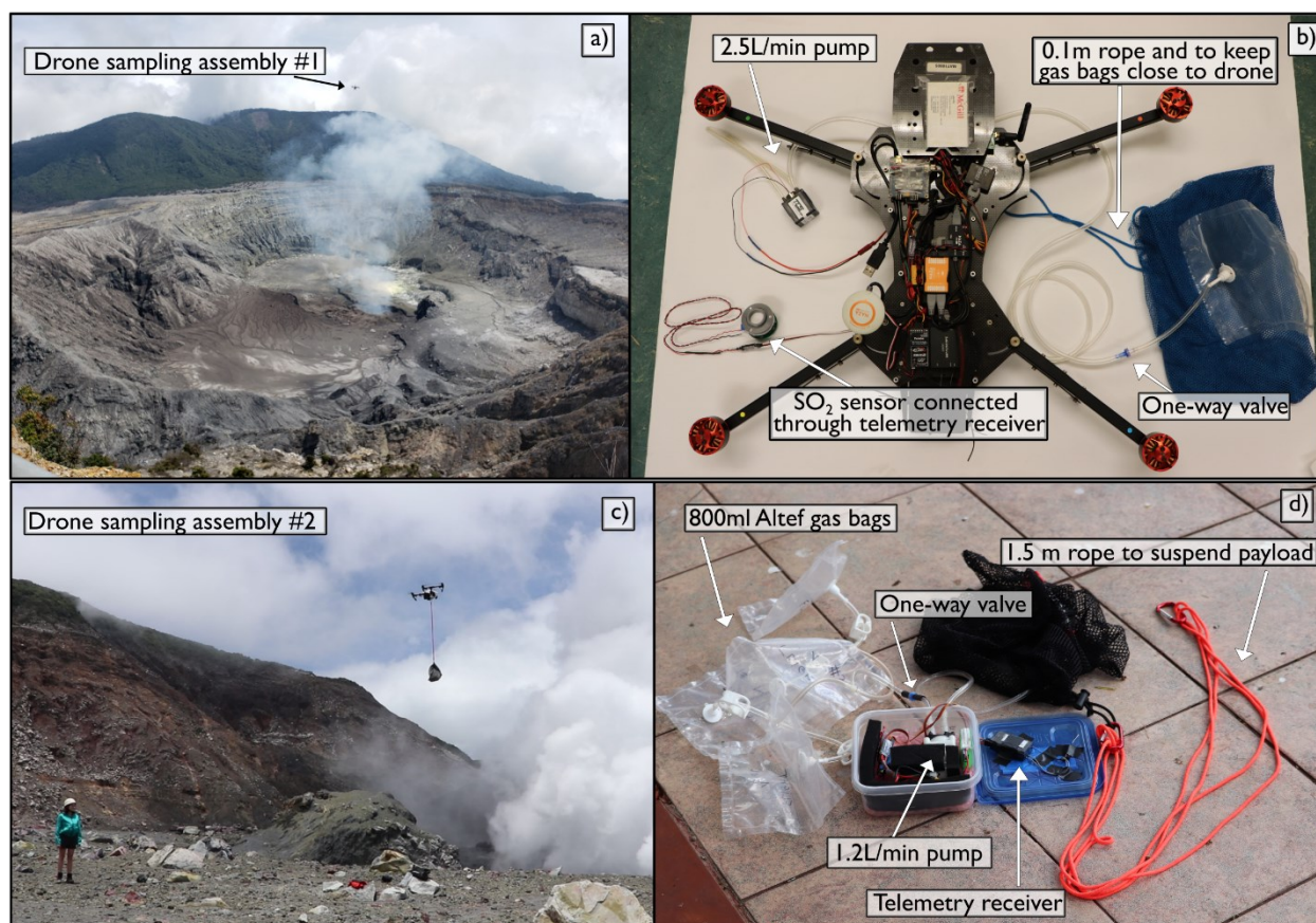
Figure 2: Sampling assembly by UAS used at Poás in April 2019. a) Distal assembly used for sampling the volcanic plume on 25 April b) Distal assembly components and specifications. c) Proximal assembly used for sampling at Poás crater on 30 April 2019. d) Proximal assembly components and specifications.
