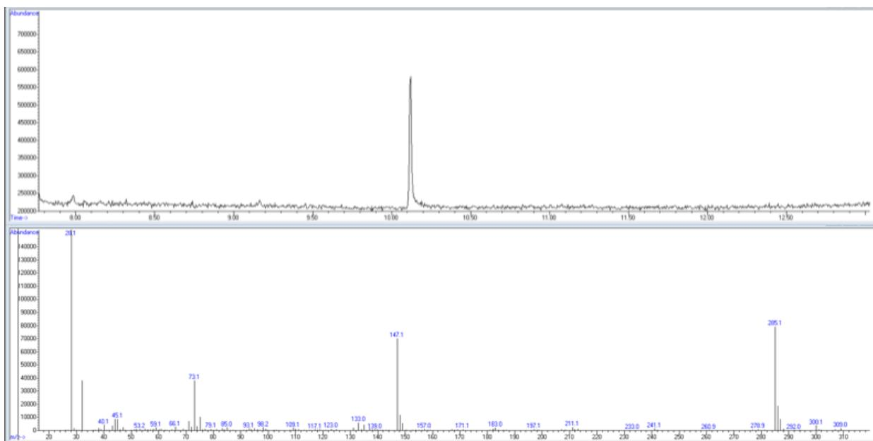
GC chromatogram and electron ionization mass spectrum of main peak from supernatant of 1 g/L HMF reaction solution with *T. reesei* whole-cells coupled with laccase/TEMPO. Library cross-reference identified this peak as 2,5-Furandicarboxylic acid, bis[trimethylsilyl] ester (the derivatized form of 2,5-furandicarboxylic acid).
