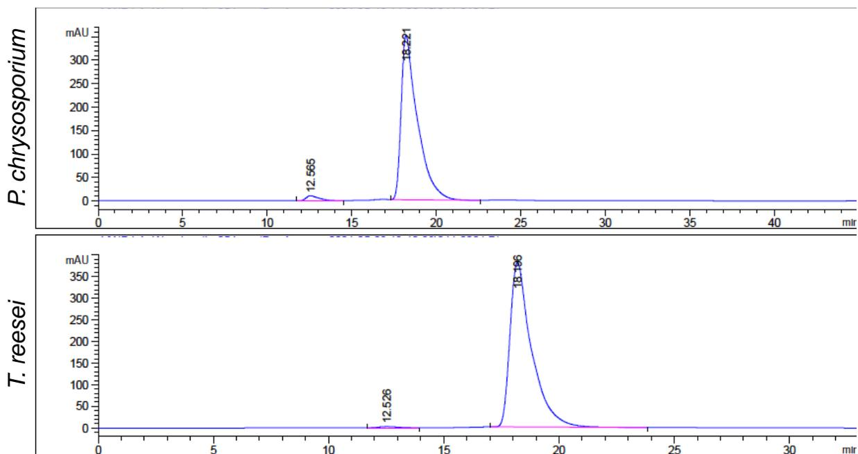
HPLC chromatograms of the supernatant from 1 g/L HMF solutions of *P. chrysosporium* (top) and *T. reesei* (bottom) following 60 hours of reaction. The main peak (RT ~ 18.2 minutes) was identified to be HMFCFA while the smaller peak (RT ~ 12.5 minutes) was identified to be FDCA. Note the different time scale when comparing chromatograms.
