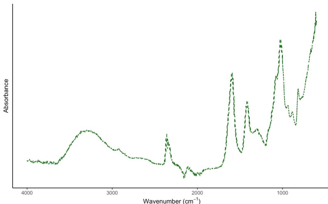
Figure S1. FTIR spectra for Ca-alginate beads without cells.
