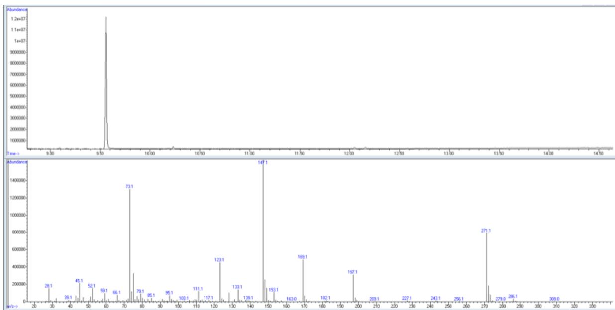
GC chromatogram and electron ionization mass spectrum of main peak from supernatant of 1 g/L HMF reaction solution with *T. reesei* whole-cells at 20-hour time point. Library cross-reference identified this peak as 2-Furancarboxylic acid, 5-[[[(trimethylsilyl)oxy)methyl]-,trimethyl ester (the derivatized form of 5-hydroxymethyl-2-furan carboxylic acid). Note: the same peak was detected as the main component in all five supernatants.
