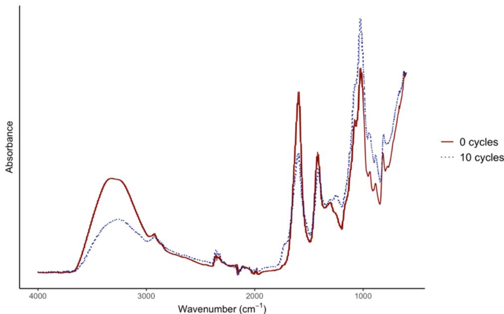
Figure 6.3. FTIR profile of the immobilized biocatalysts prior to any reactions and after 10 reuses (red solid line and blue dashed line respectively).
