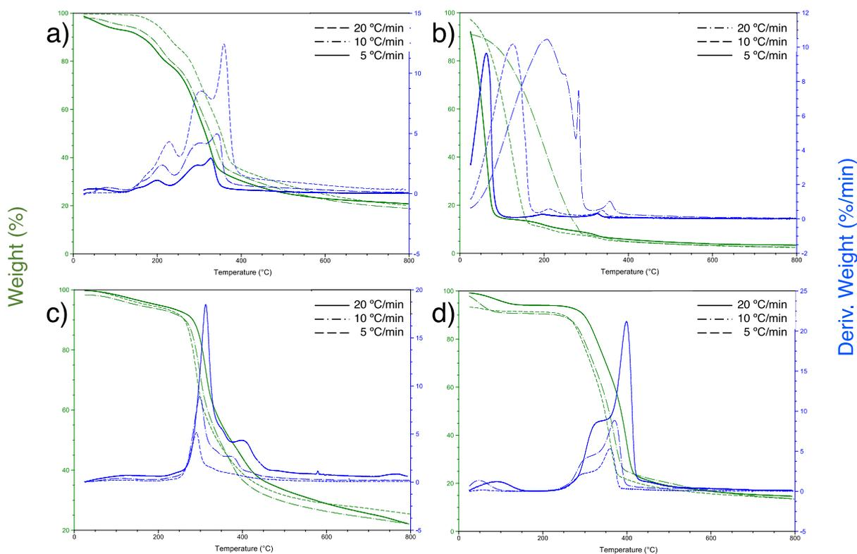
Figure S1. Method optimization for thermogravimetric analysis. Results of change in weight at heating rates of 20, 10, and 5 °C/min are shown for: a) corn cob; b) apple pomace; c) simulated food waste; d) hardwood.
