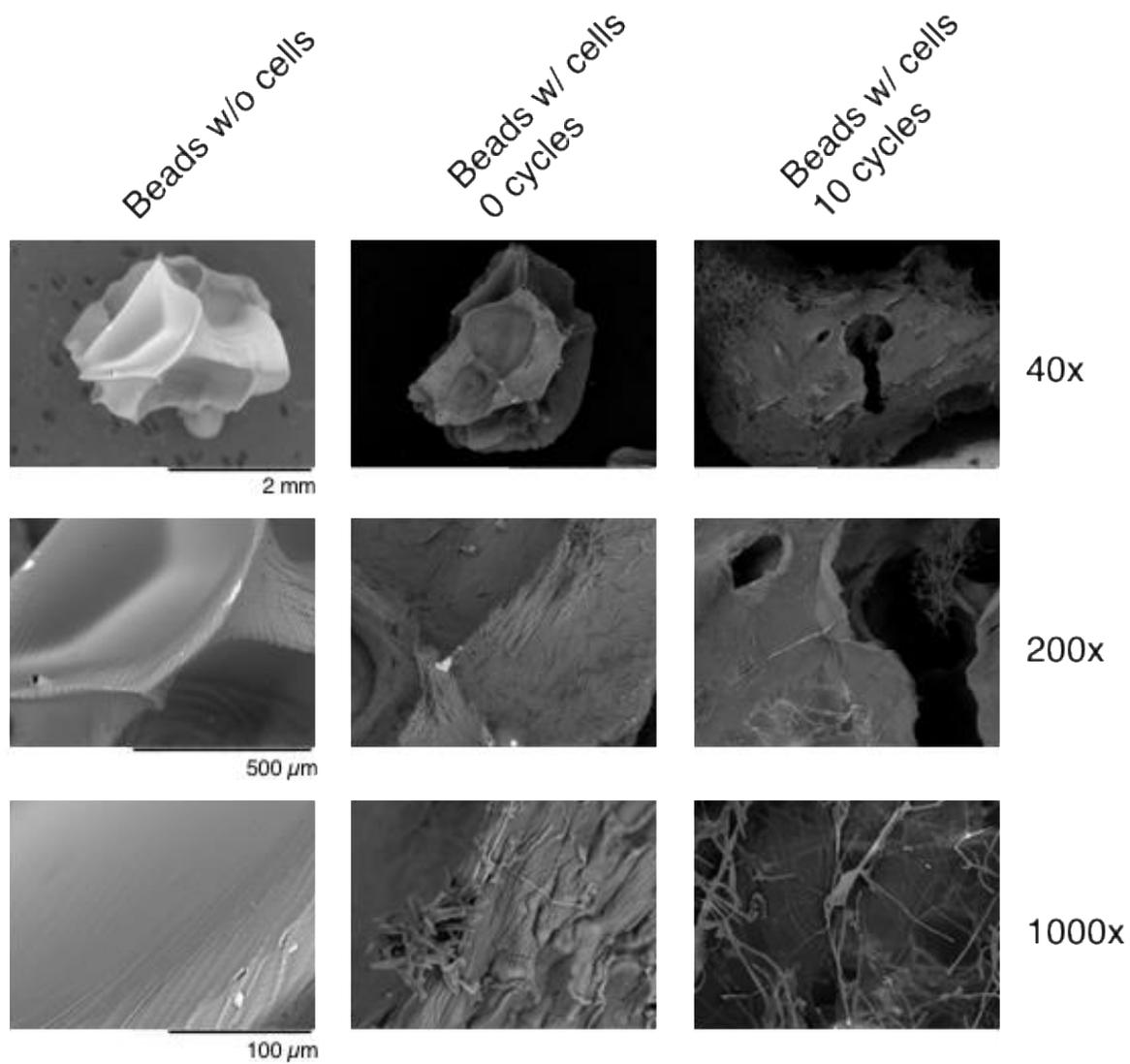
Figure 6.2. SEM images at increasing magnification of the surfaces of calcium alginate beads without any cells (first column) and the immobilized biocatalysts prior to any reactions and after 10 reuses (second and third column respectively).
