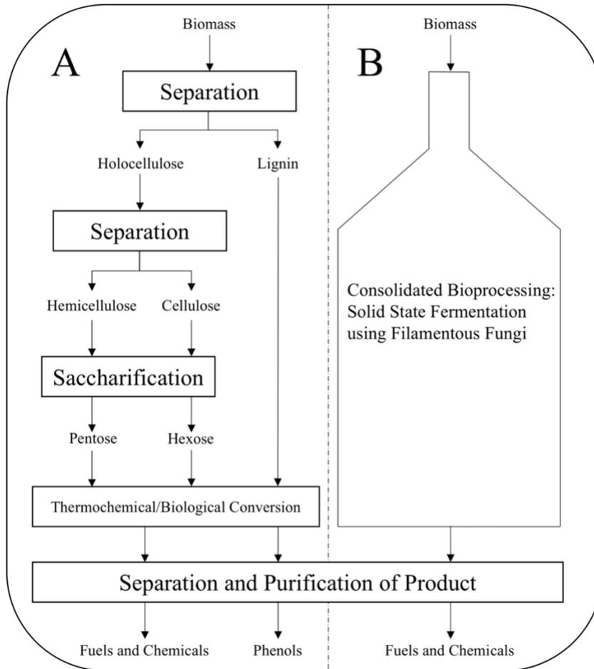
Fig. 2.4. (A) represents a typical process flow of raw biomass to final products while (B) represents a theoretical consolidated bioprocess, in this scenario using fermentation via filamentous fungi, where many of the original process steps are condensed into one step.
