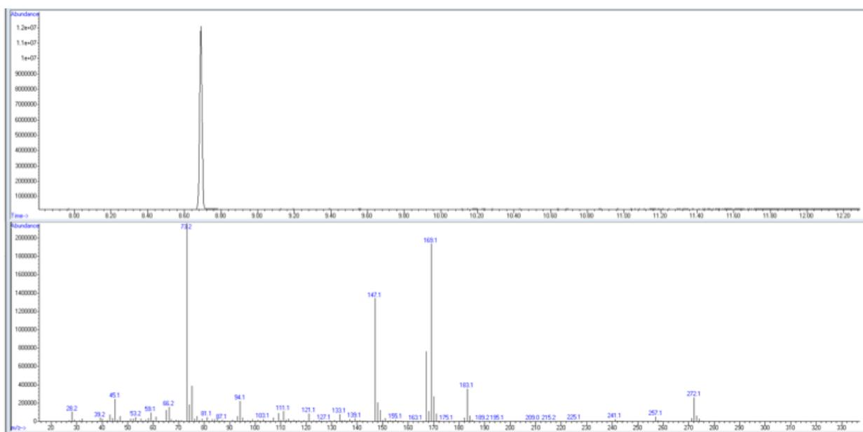
GC chromatogram and electron ionization mass spectrum of main peak from *P. purpurogenum* cell homogenate of 1 g/L HMF reaction solution. Library cross-reference identified this peak as 2-Furanacetic acid, alpha-[(trimethylsilyl)oxy]-,trimethyl ester (the derivatized form of Furan acetic acid)
