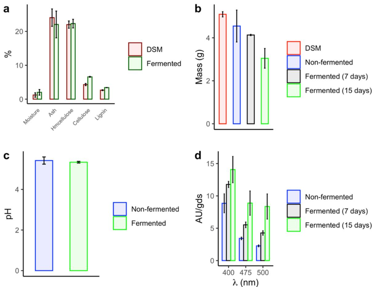
Figure 4.1. a) Summary of results of thermogravimetric, acid detergent fiber, neutral detergent fiber, and lignin detergent fiber analyses of SFW dry starting matter (DSM) and fermented SFW. Note: The values from detergent fiber analyses (hemicellulose, cellulose, and lignin) are on a dry matter basis; b)
