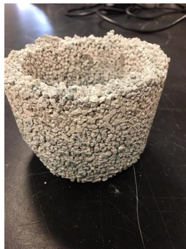
Figure 16 – Properly cured Quartz sample
