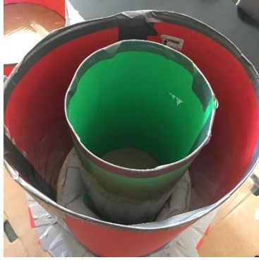
Figure 19 – Mold for body,
