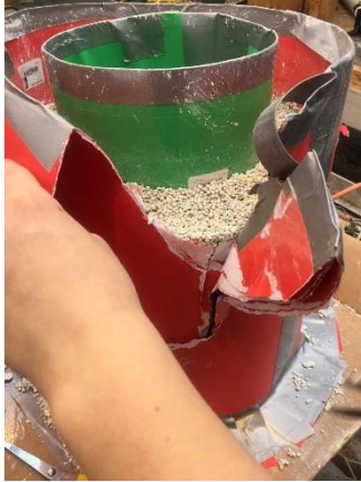
Figure 23 – Easy unmolding of body
