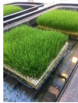
Figure 2 – Porous Concrete supporting plants
