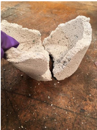
Figure 15 – Fractured sample after curing
