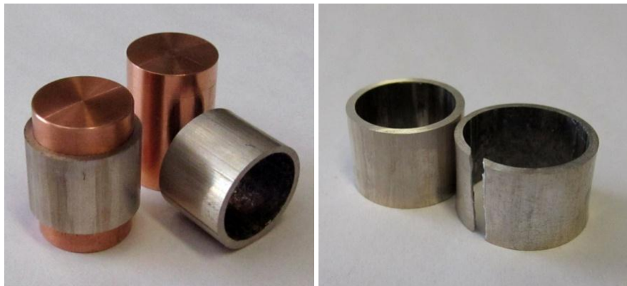
Figure .7.2.3. (a) Copper insert and magnesium tube assembly before deformation, (b) magnesium tubes before and after deformation.
