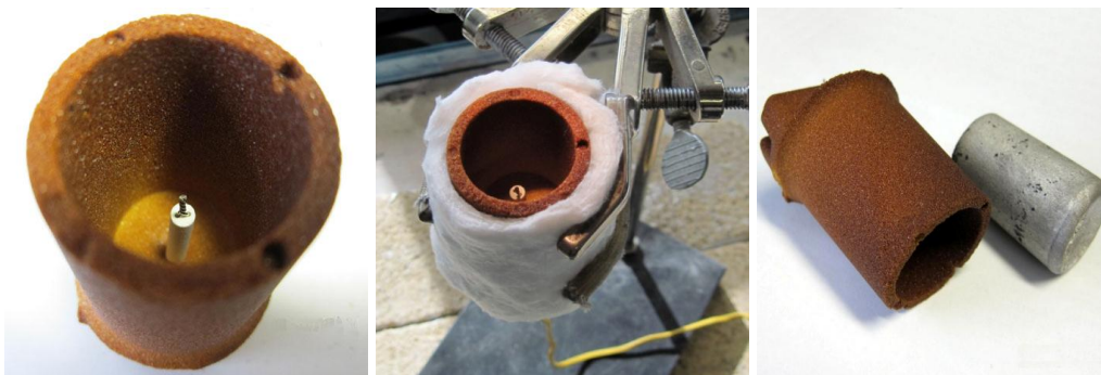
Figure.3.1.1. (a) a sand cup with a fixed exposed junction thermocouple, (b) an installed sand cup ready for casting, and (c) the cast sample after solidification.
