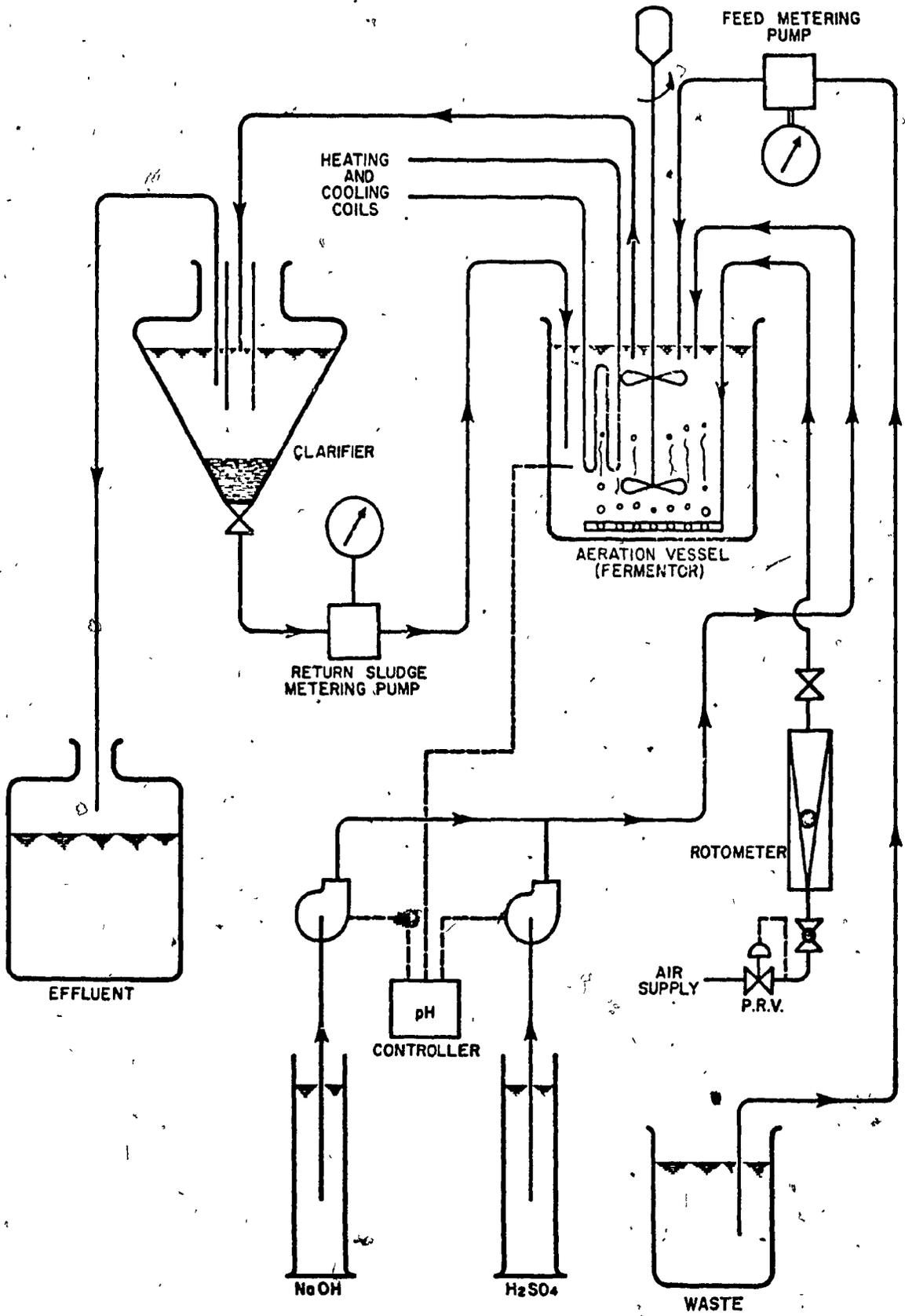
controller (model pH-22) within  $\pm 0.3$  of the preset value on the pH-scale.
