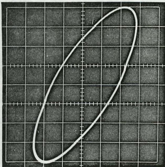
Fig. 315. Terminal voltage vs. current at 60 cps. Scale 10 v/square, 7 ma/square. No d-c. Terminal admittance 0.465 millimhos, phase angle  $-40^\circ$ .
