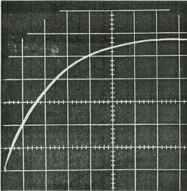
Fig. 306. Current through d-c machine armature and interpoles in response to a voltage step. 5 amp/square, 5 msec/square.
