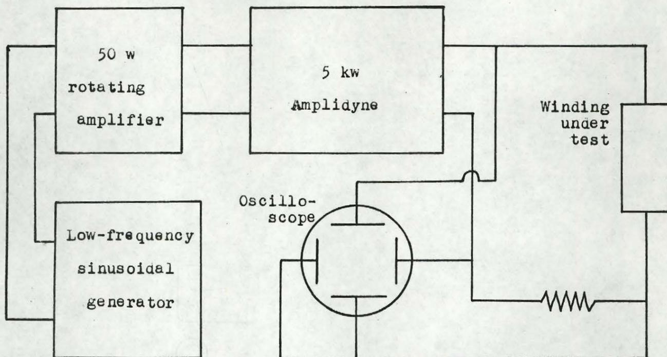
Fig. 314. Equipment layout for measurement of incremental admittance magnitude and angle at low frequencies. The d-c source exciting a second input winding of the amplidyne is not shown.
