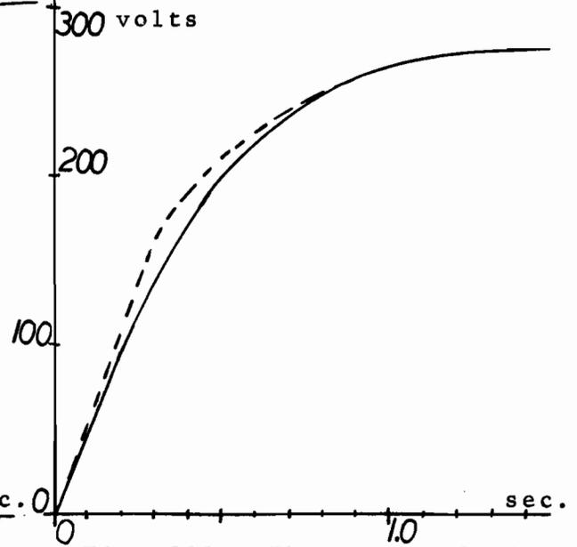
Fig. 311. The curve of Fig. 308, showing predicted and measured open-circuit voltage.
