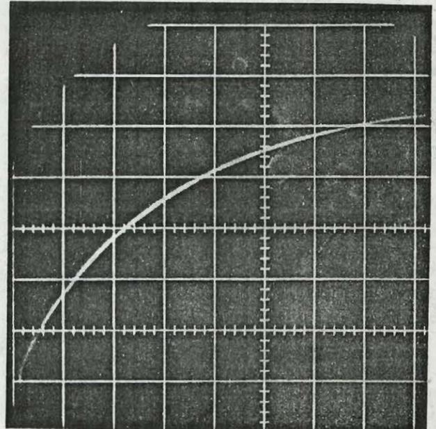
Fig. 307. Current through d-c machine armature alone, in response to a voltage stepfunction. 2.5 amp/square, 2 msec/square.
