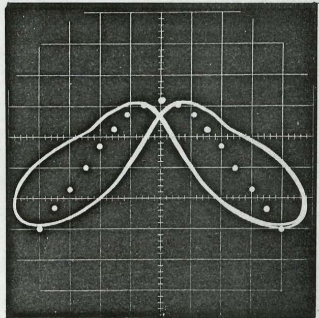
Fig. 503. Stator current (horizontal) vs. rotor terminal voltage (vertical). Rotor direct current 1.5 amperes. Dots represent predicted points.
