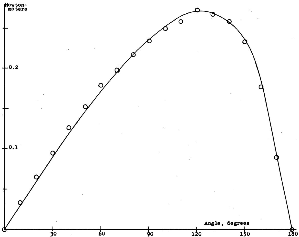
Fig. 507. Shaft torque against rotor position for the test machine. Rotor current 1.19 amperes, stator current 1.19 amperes. Solid line represents predicted, circles experimental points.
