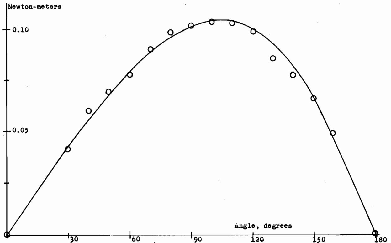
Fig. 506. Shaft torque against rotor position for the test machine with rotor current 1.19 ampere, stator current 0.40 ampere. Solid line represents predicted, circles experimental values.
