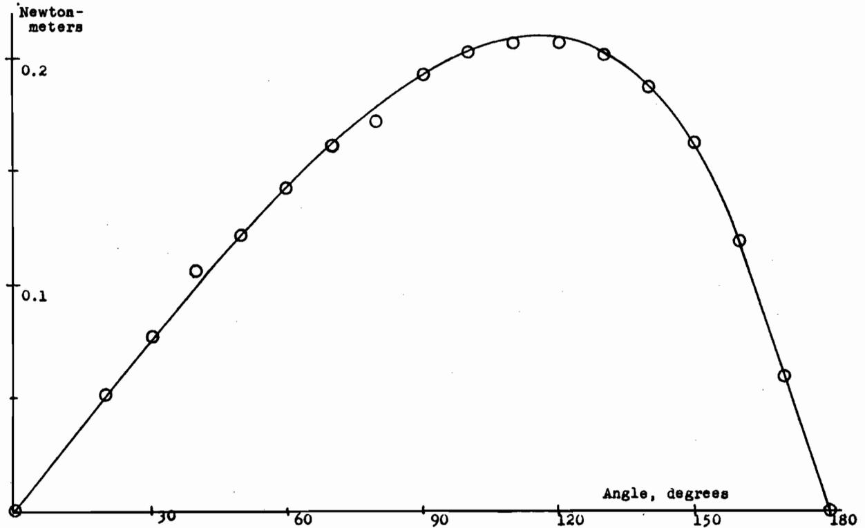
Fig. 505. Shaft torque against rotor position of the test machine with rotor current 1.19 ampere, stator current 0.76 ampere. Solid line represents predicted, circles experimental values.
