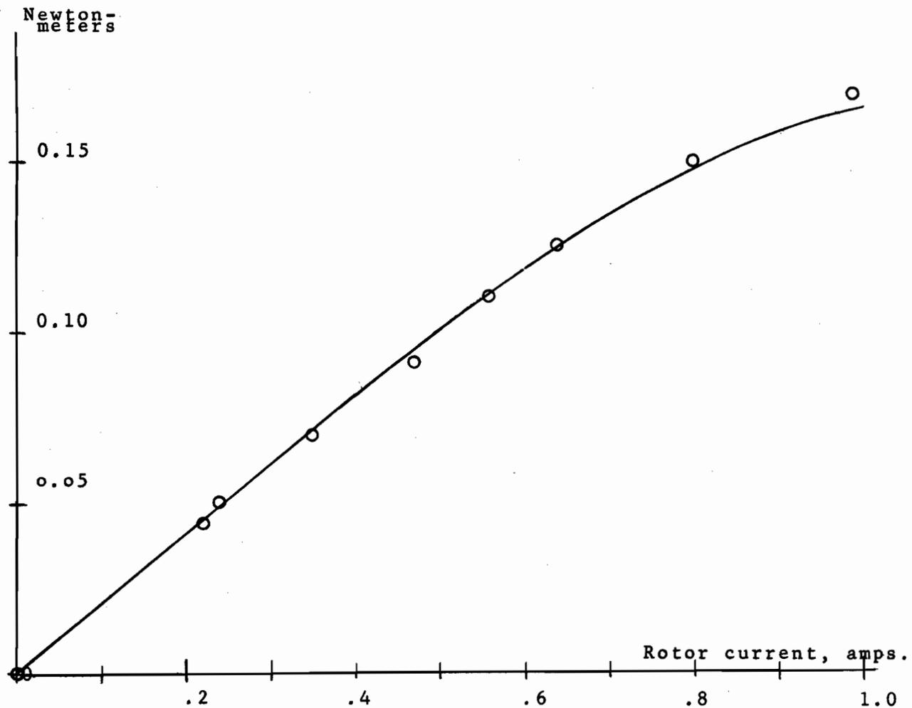
Fig. 509. Shaft torque of the test machine against the rotor current, with stator current held constant at 0.70 ampere and the rotor position at  $120^{\circ}$ . Solid line represents predicted, circles experimental values.
