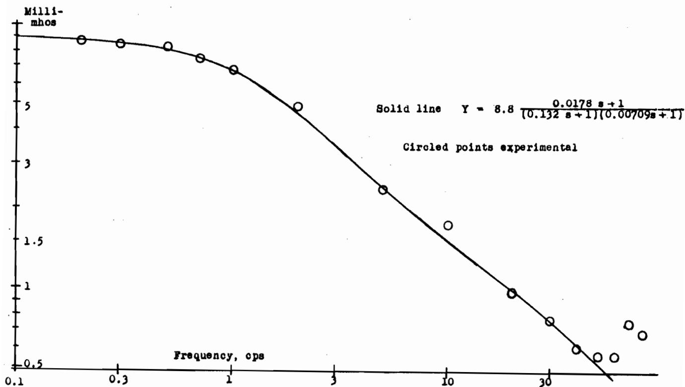
Fig. 320. Behaviour of incremental field admittance with frequency, at the rated value of d-c field current ( 1.0 ampere ).
