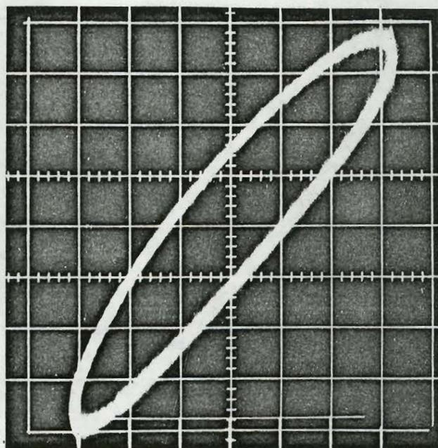
Fig. 316. As Fig. 315, but at 0.7 cps and a d-c current component of 0.9 amp. Note asymmetry arising from nonlinearity. Current scale 38 ma/square, admittance  $7.08 / -22^\circ$  millimhos.
