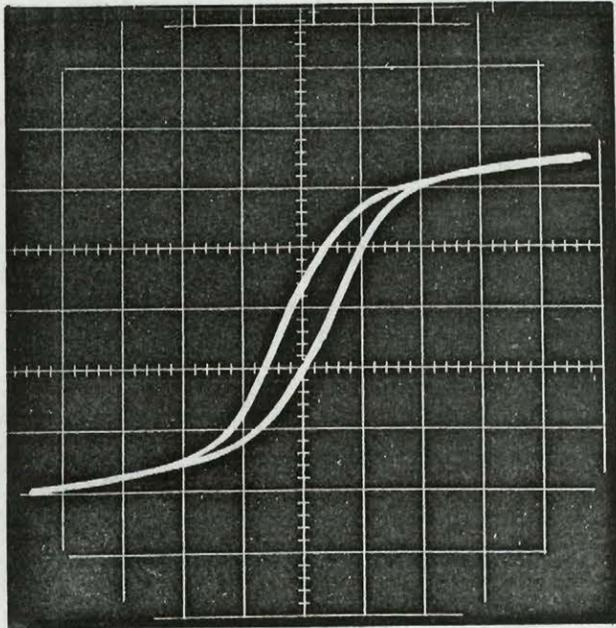
Fig. 502. Dynamic hysteresis loop of test machine, with rotor energised at 30 cps. The rotor peak current is 2.3 amperes.
