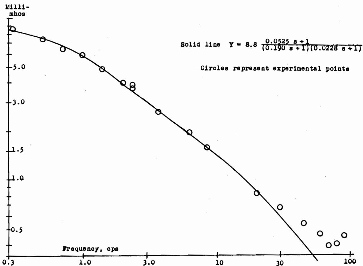
Fig. 319. Behaviour of incremental field admittance with frequency, with d-c field current of 0.75 ampere.
