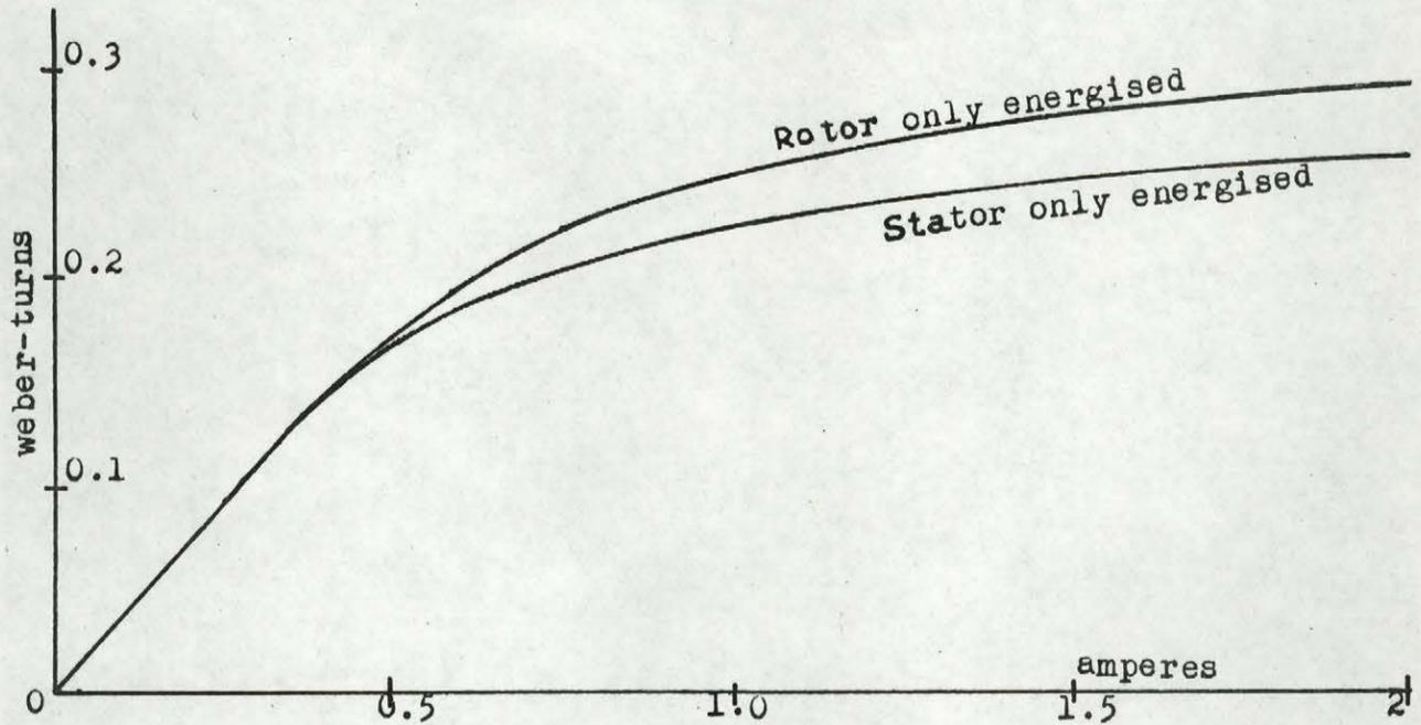
Fig. 501. Static mean magnetisation curve of the test machine, measured by energising only one winding at a time and finding flux linkages of the other.
