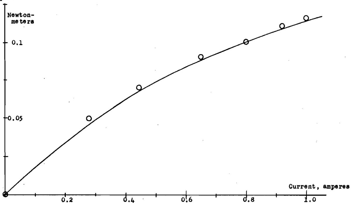
Fig. 508. Shaft torque of the test machine against rotor current, with stator current held constant at 0.70 ampere and rotor position at 58°. Circles represent measured points, solid line predicted values.
