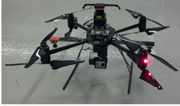
Figure 5–5: The Draganflyer X8 retrofitted with LIDAR, beam directing mirrors and a GoPro camera.
