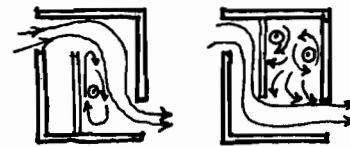
Fig. 1.18 Indoor air flow affected by partitions (Source: Konya, 1980, p.53)
