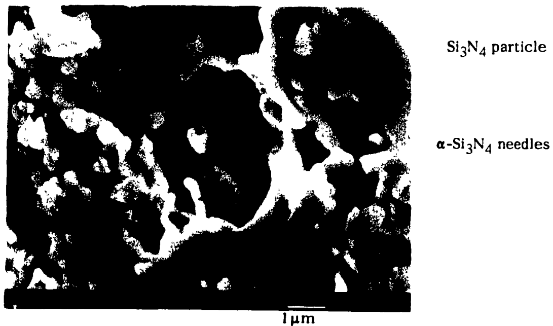
Fig 5.19: \alpha - \text{Si}_3\text{N}_4 needles in a pore.
