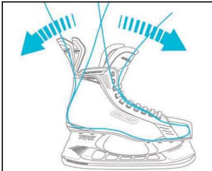
Figure 10: Modified skate with a flexible tendon guard to increase range of motion (adapted from: [www.bauer.com](http://www.bauer.com)). Figure shown is of a different skate model but the same concept is applied to the modified skate being used in this study.)
