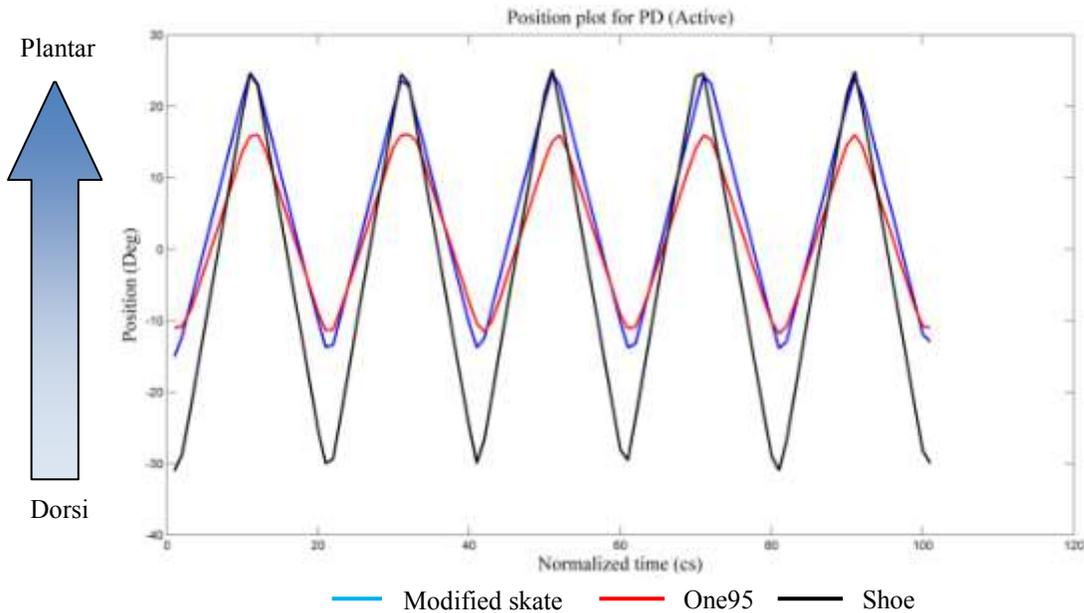
**Figure 13: Sample trial of angular position (and ROM) for each footwear condition. Greatest ROM was found in the shoe, and least in the One95 skate.**
