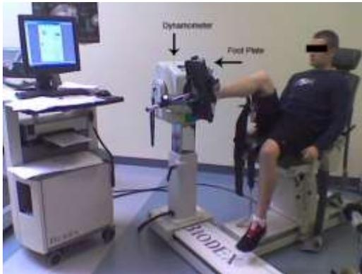
Figure 6: Biodex Dynamometer set-up
