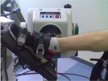
Figure 1: Side view of the ankle foot complex in plantar-flexion, set up in the Biodex Dynamometer
