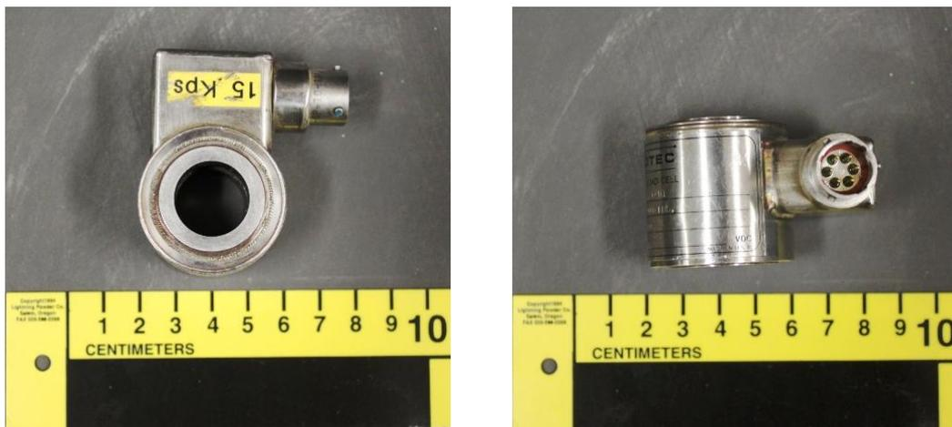
Figure A - 5: Sensotec 67 kN (15 kips) donut load cell
