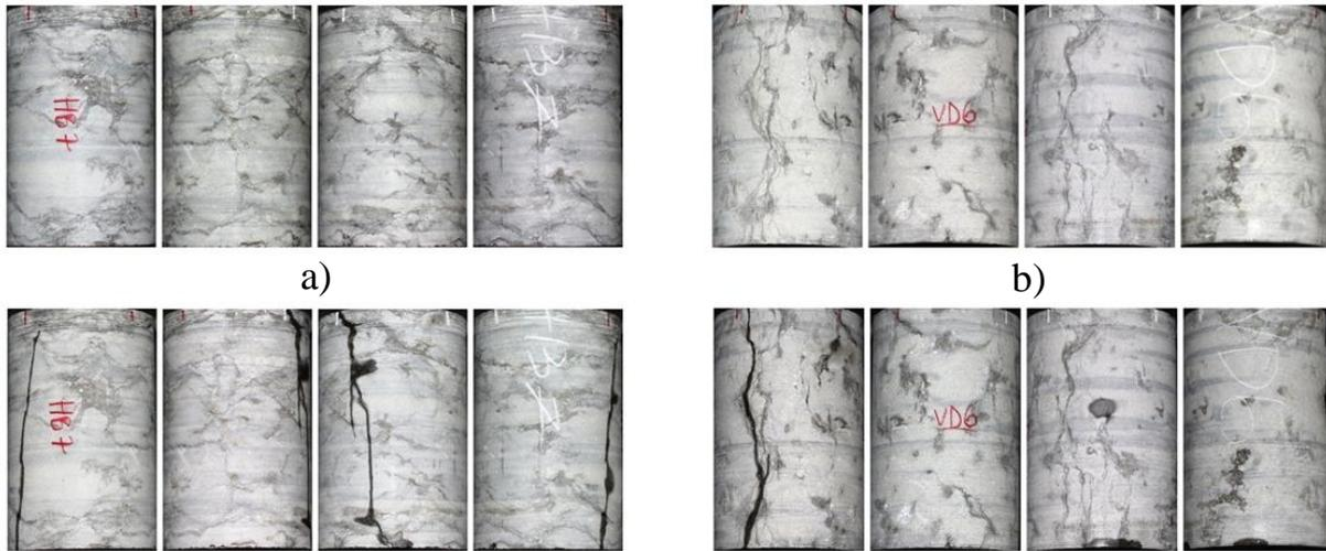
Figure 28: Typical failure patterns of the plug compression test samples
