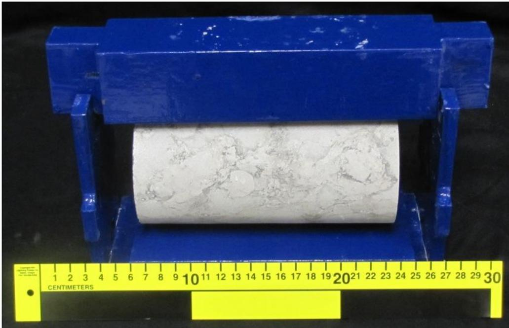
Figure 23: Brazilian splitting test apparatus with LCL cylinder
