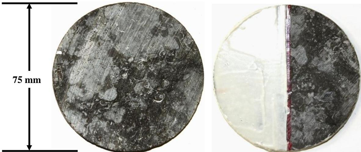
Figure 7: Thin Disks of Lindsay Cobourg Limestone; a) full disk, b) half disk sealed with marine epoxy
