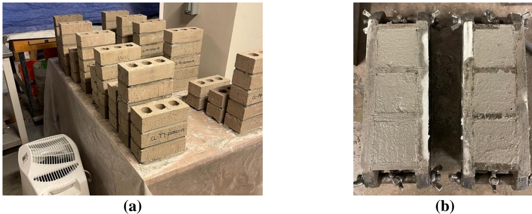
Figure 7. (a) Clay brick doublets, triplets, and prisms; (b) Type N mortar cubes
