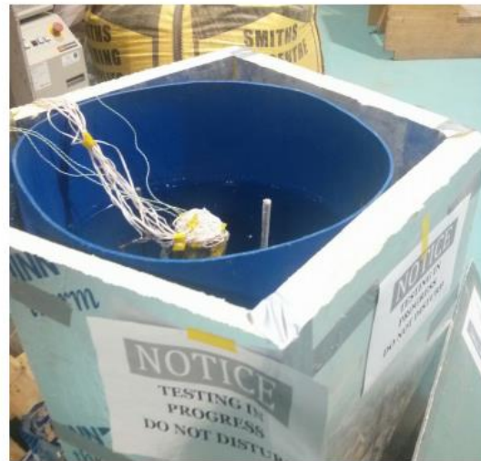
(b) Photograph of 76.2 mm sample in the water bath
