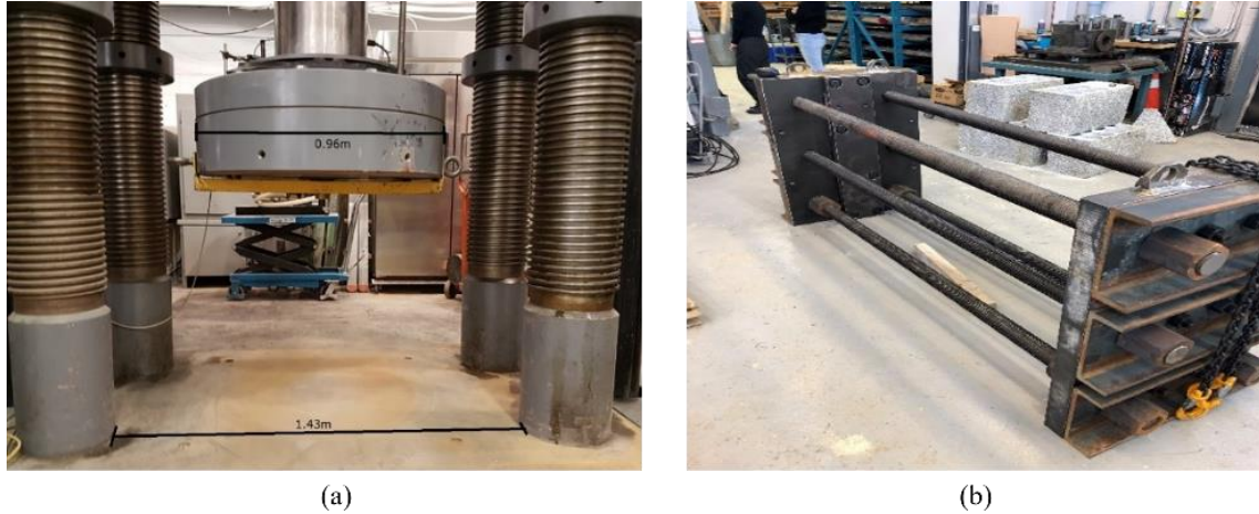
Figure 4.2: Biaxial loading test apparatus, (a) Vertical press, b) Lateral loading frame.
