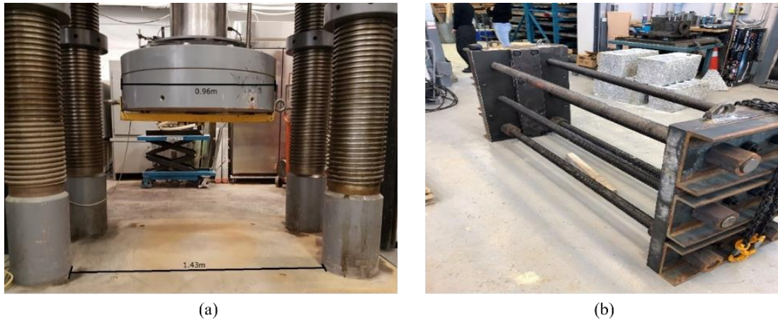
Figure 3.13: Biaxial loading test apparatus, (a) Vertical press, b) Lateral loading frame.
