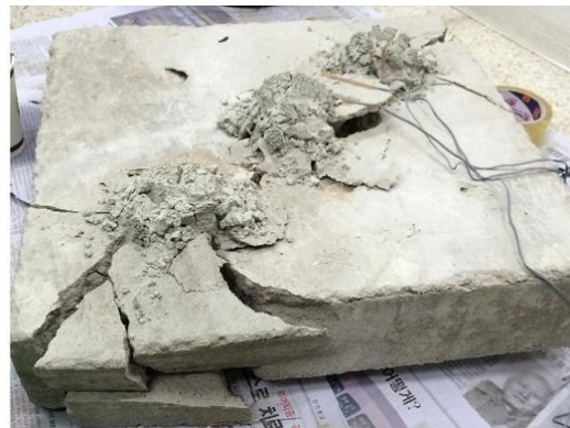
(b) Concrete demolition with EC
