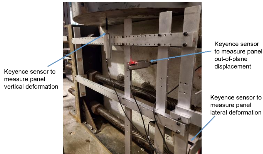
Figure 4.5: The location of purpose of Keyence sensors.
