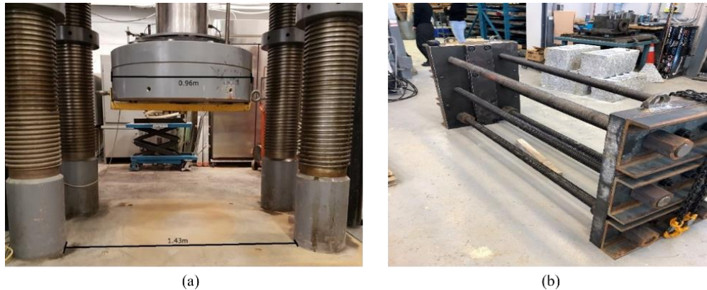
Figure 5.3: Biaxial loading system, a) Vertical press, b) Lateral loading frame (Chen et al., 2022).
