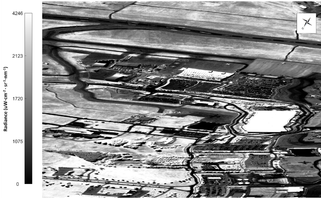
Figure 3.22. Histogram-equalized CASI imagery (24 June with original processing) at 931.099 nm. The imagery is stable, with no obvious errors.
