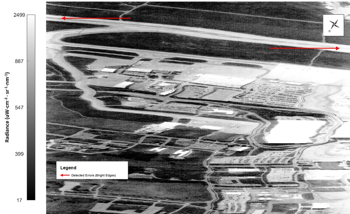
Figure 3.14. Histogram-equalized CASI image (24 June with the original processing) at 393.068 nm. The asphalt road along the south side of the image was brightest along the edge pixels. The errors in the data are highlighted by the red arrows.
