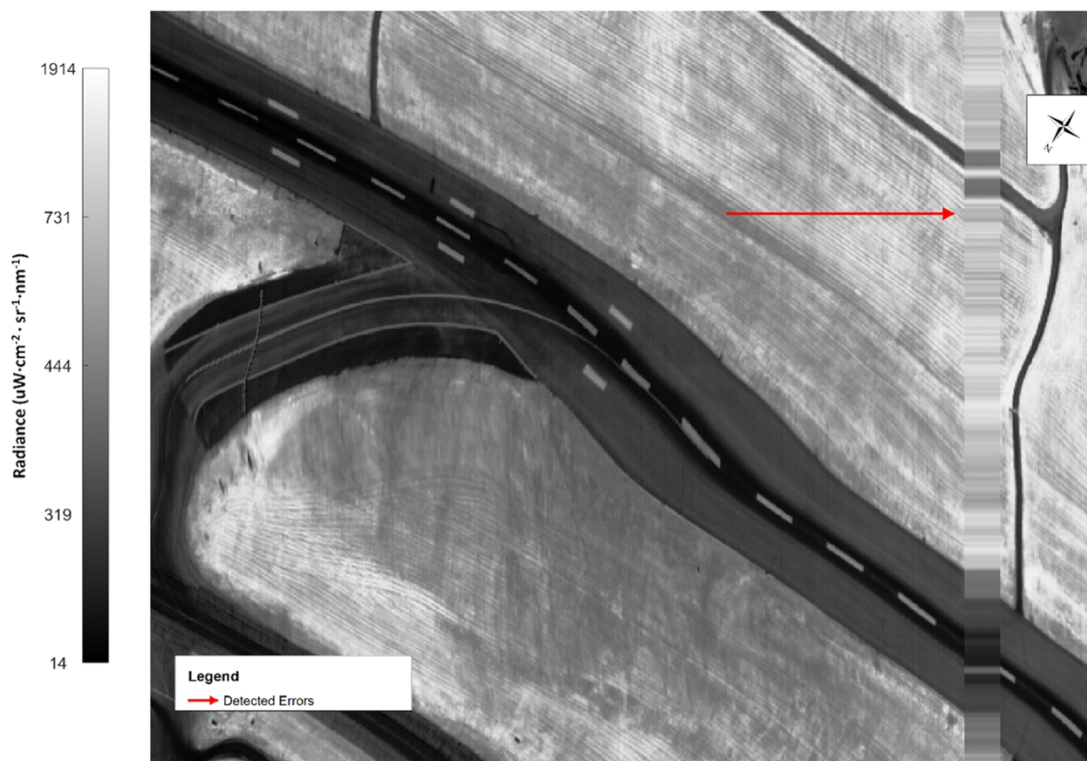
Figure 3.16. Histogram-equalized SASI imagery (24 June with the refined processing) at 1003 nm. An error across Pixels 548–564 is identified by the red arrow.
