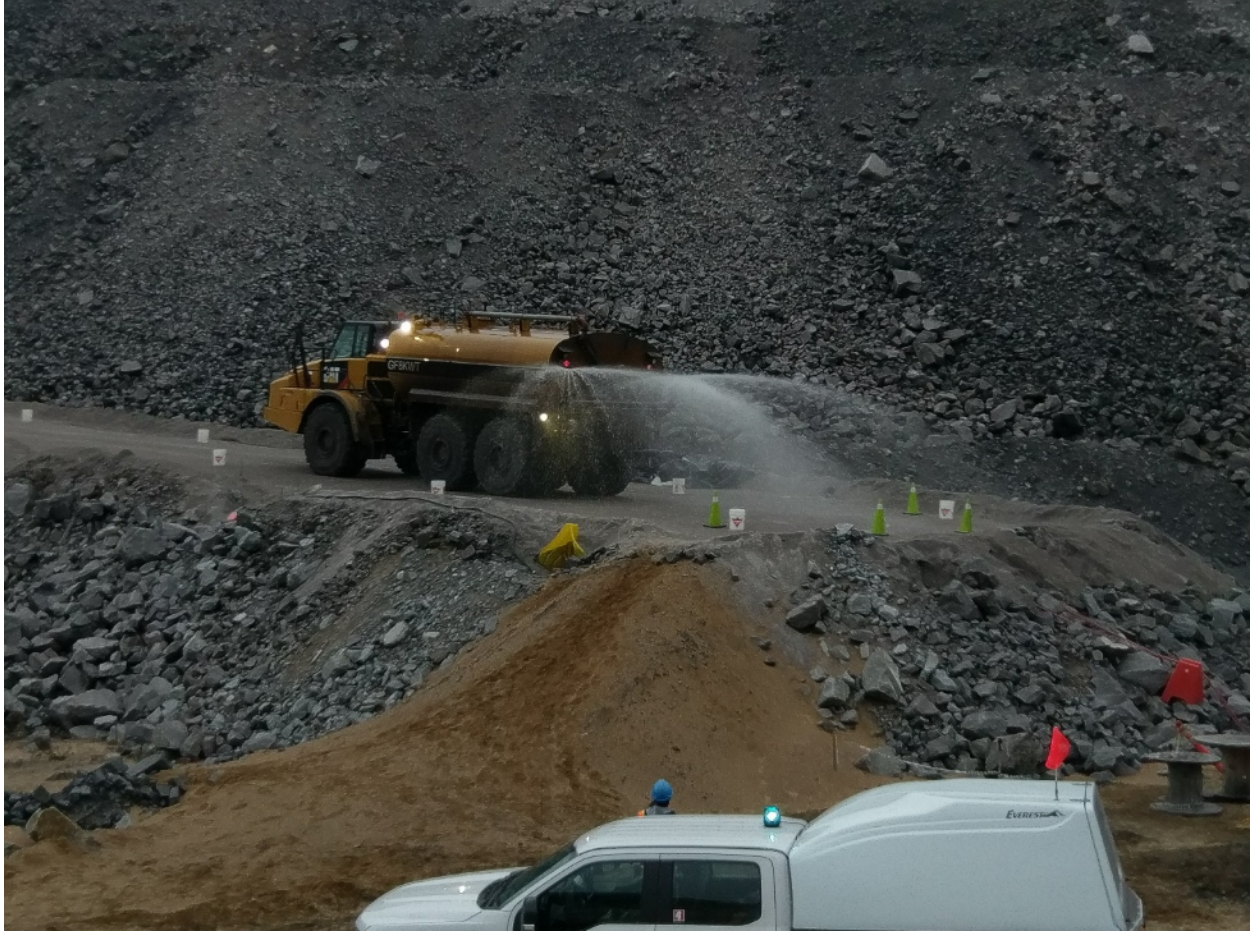
Figure 3.3: Artificial precipitation was applied with a water truck to simulate short duration, large volume precipitation events.
