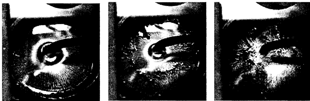
Figure 56 – Formation of an apparently solid oxide on Pb-0.9 wt% As molten alloy surface by impingement of oxygen gas.
