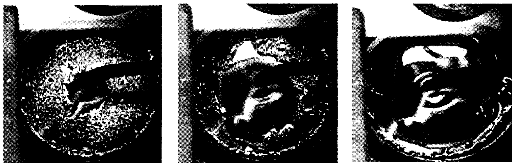
Figure 57 – Disappearance (melting) of the solid oxide layer on the surface of Pb-0.9 wt% As molten alloy by the flow of the argon gas on the surface of the melt.
