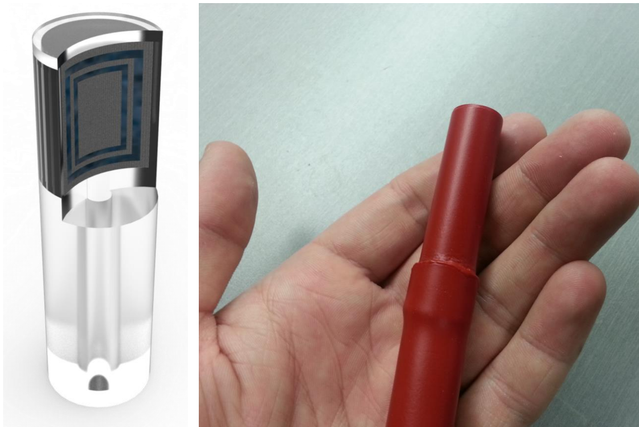
Figure 4.2: (Left) An isometric view of a cutaway GPC rendering, with the layers of aerogel-based thermal insulation seen between the three graphite bodies. The graphite assembly is housed in an acrylic stem. (Right) The GPC-MKIV prototype was designed to be similar in size and shape to a 0.6 cm 3 cylindrical ionization chamber, and used in the radiation therapy clinic in much the same way.
