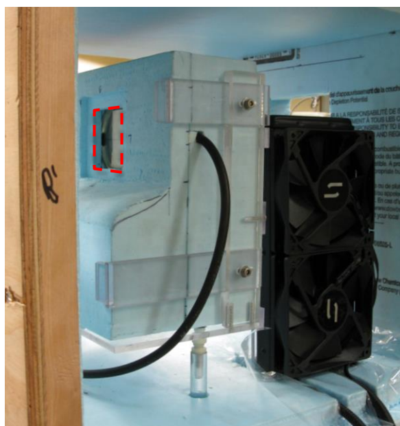
Figure 7.4: Photographs of the SHREWcal as seen from (top) the side with one wall removed, (bottom left) the side with the vessel window outlined by a red dashed line, and (bottom right) from the beam's eye point of view.
