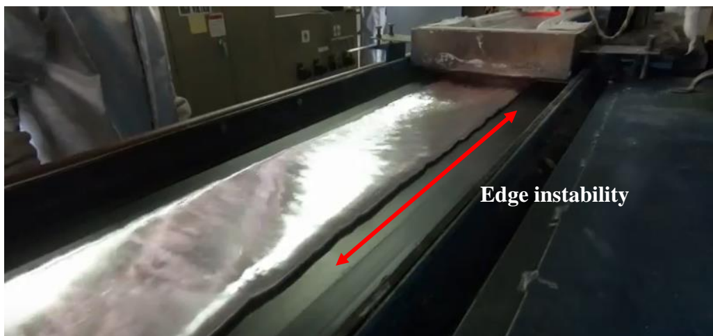
Figure 4-8 Edge instability produced by downstream disturbance
