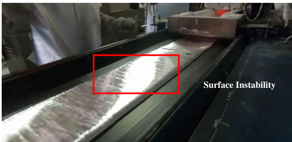
Figure 4-8 Edge instability produced by downstream disturbance
