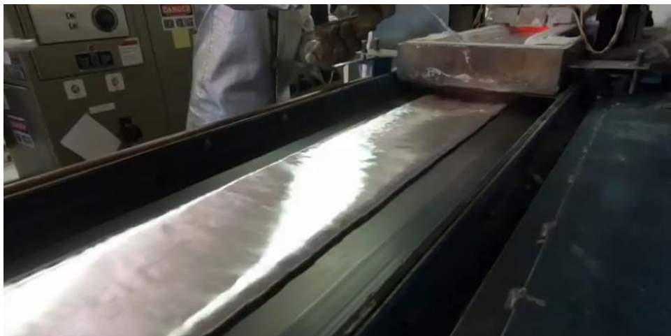
Figure 4-7 280 mm AA2024 strip during casting using the HSBC pilot-scale machine
