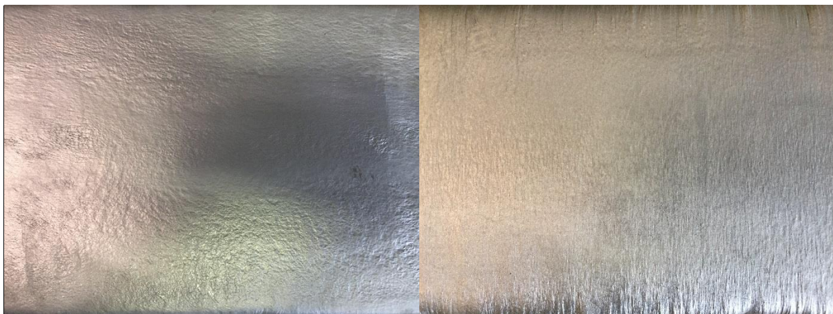
Figure 4-10 180 mm wide strip top surface (Left) and 200 mm wide strip top surface (Right), with casting direction from left to right
