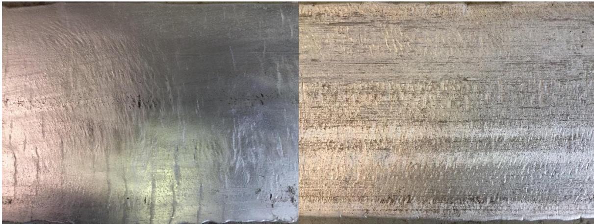
Figure 4-11 180 mm wide strip bottom surface (Left) and 200 mm wide strip bottom surface (Right), with casting direction from left to right
