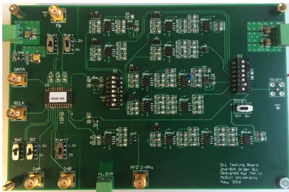
Fig. 5.2: Front view of DLL testing PCB.
