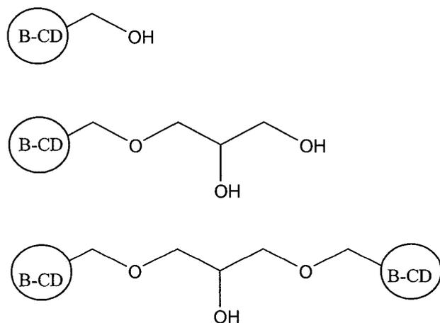
**Figure 6.2** Suggested molecular structures of  $\beta$ -CD-EP polymer obtained from the polymerization reaction (For simplicity, only reactions on primary alcohols are shown.)
