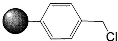
**Figure 1.1** – Merrifield resin (O- represents polystyrene backbone)
