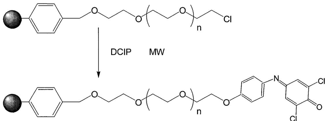
**Scheme 5.2** Microwave assisted immobilization of DCIP to thionyl chloride activated PEGylated MR.
