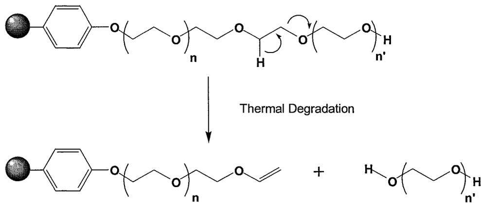
**Scheme 3.3** Thermal degradation of PEGylated Merrifield resin based on pyrolysis-GC/MS analysis.
