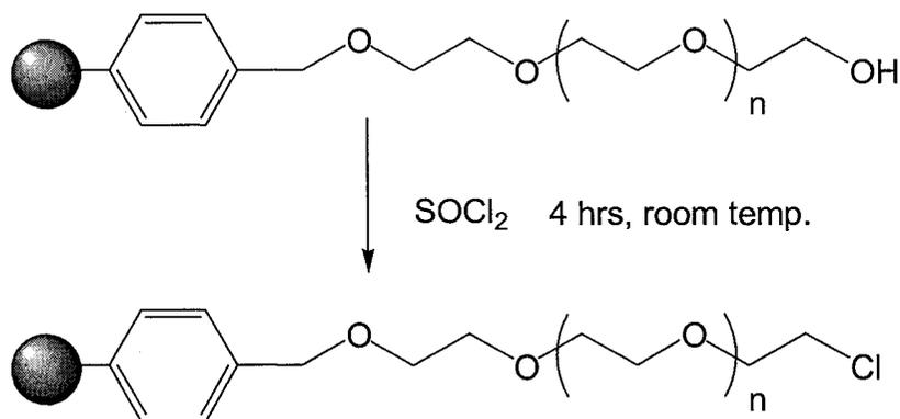
**Scheme 4.2** Substitution of the hydroxyl group of PEG using thionyl chloride
