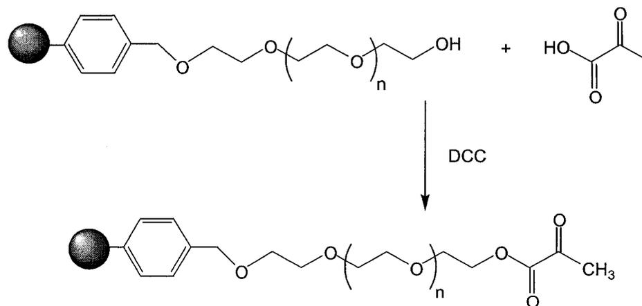
**Scheme 4.1** Esterification of PEGylated Merrifield resin with pyruvic acid
