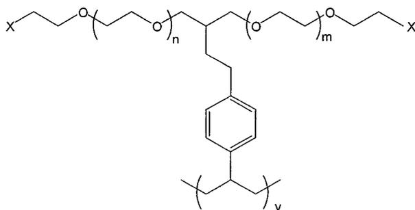
**Figure 2.2** AgroGel - new graft-type PEG-PS with twice the loading capacity of TentaGel
