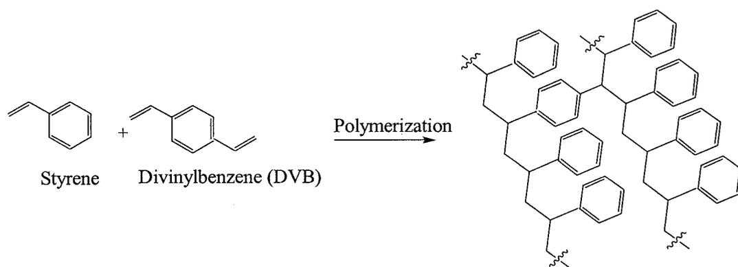
**Figure 1.2** – Suspension polymerization of polystyrene resin
