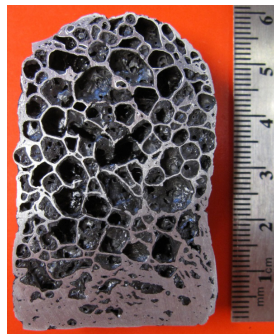
Figure 5.62: Al-99.99 / \text{Al}_2\text{O}_3 foamed to maximum expansion at 800°C
