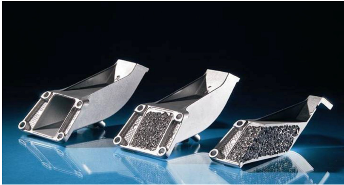
Figure 2.8: BMW engine mounting bracket prototype, before aluminum foam filling (left), after foam filling (middle) and sectioned (right)
