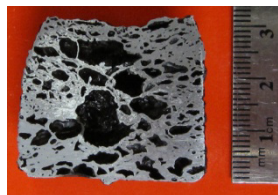
Figure 5.101: Al-7Cu / SiC foam overaged at 729°C
