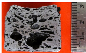
Figure 5.100: Al-7Cu / SiC foamed to maximum expansion at 729°C
