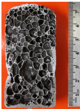
Figure 5.106: Al-1Mg / SiC foamed to maximum expansion at 798°C
