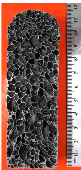
Figure 5.78: A356 / \text{Al}_2\text{O}_3 foamed to maximum expansion at 764°C
