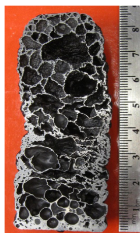
Figure 5.79: A356 / \text{Al}_2\text{O}_3 foam overaged at 764°C
