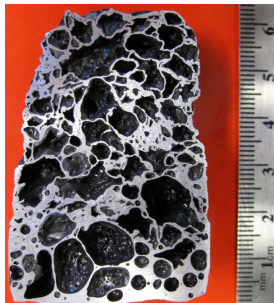
Figure 5.69: Al-7Cu / \text{Al}_2\text{O}_3 foam overaged at 729°C
