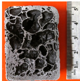
Figure 5.105: Al-1Mg / SiC foam overaged at 748°C
