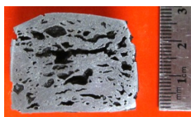
Figure 5.96: Al-11.5Si / SiC foamed to maximum expansion at 688°C
