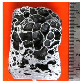
Figure 5.94: Al-99.99 / SiC foamed to maximum expansion at 800°C
