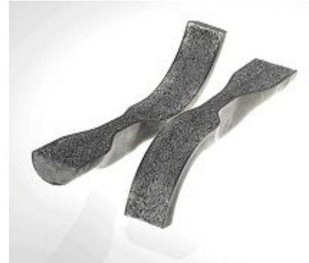
Figure 2.4: Steel profile filled with aluminum foam made via the PM method
