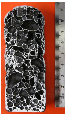
Figure 5.77: A356 / \text{Al}_2\text{O}_3 foam overaged at 714°C
