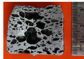
Figure 5.103: Al-7Cu / SiC foam overaged at 779°C
