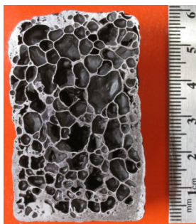
Figure 5.104: Al-1Mg / SiC foamed to maximum expansion at 748°C
