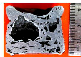
Figure 5.99: Al-11.5Si / SiC foam overaged at 738°C
