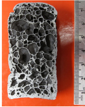
Figure 5.81: AA6061 / \text{Al}_2\text{O}_3 foam overaged at 754°C
