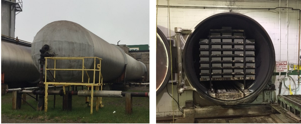
Figure 3.13: Autoclaves or pressure vessels traditionally used to cure the CMU's at Boehmers
