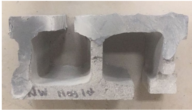
Figure 3.15: Sawn surfaces for phenolphthalein and pH tests
