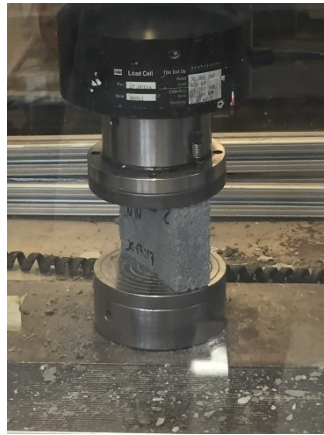
Figure 3.8: Slabs compressed along weak axis using an MTS Sintech machine
