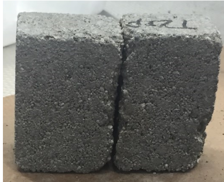
Figure 3.9: Sawn surfaces of laboratory slabs for phenolphthalein and pH tests
