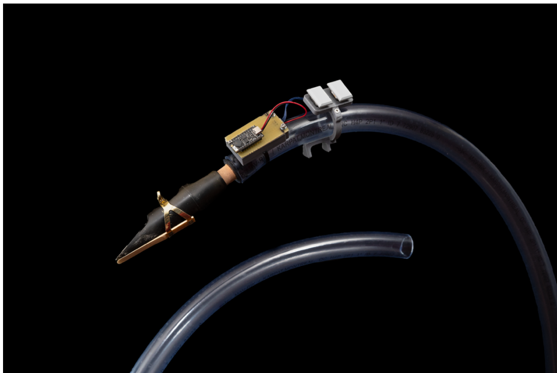
Fig. 5.7: The eTube gamma version with baritone saxophone mouthpiece.
