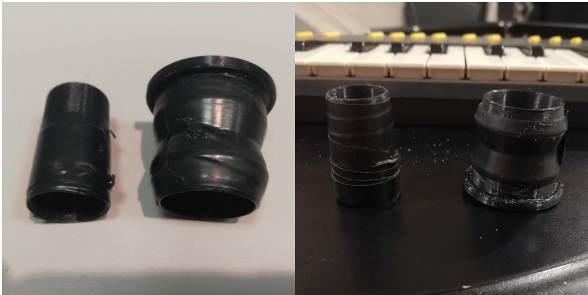
Fig. 3.6: The mouthpiece adapters would often break in the same place.
