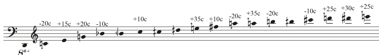
Fig. 3.8: The overtones accessible by overblowing a 2.54 cm diameter, 219 cm long eTube with a baritone saxophone mouthpiece, transcribed by Quentin Lauvray.
