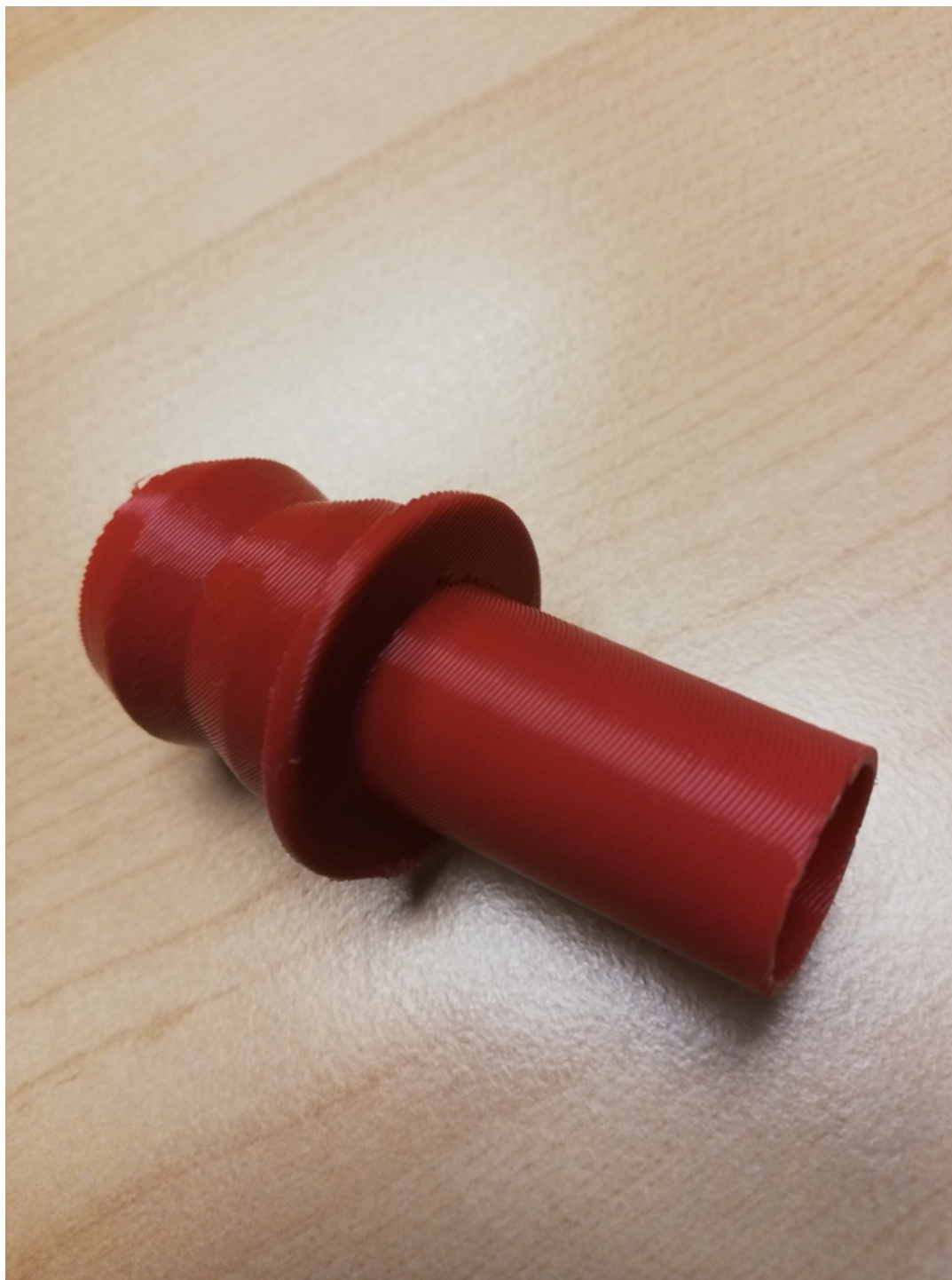
Fig. 3.7: This baritone saxophone mouthpiece adapter was 3D-printed at a 45-degree angle.
