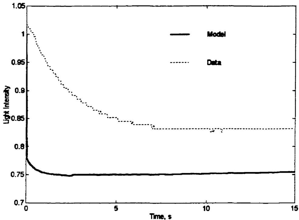
**Figure 4.10 Calculated and measured reflection intensity. The incident angle for the model execution was 30°.**
