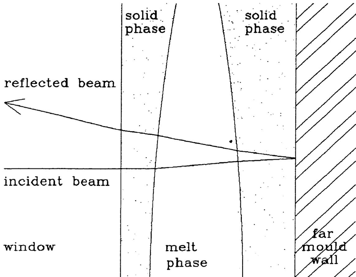
**Figure 4.11 Approximation to the path of the laser beam inside the mould cavity during solidification**
