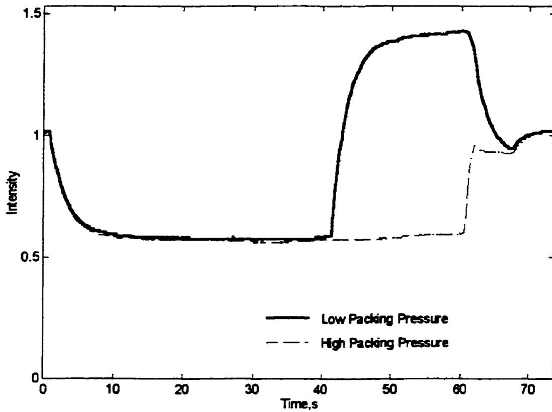
**Figure 4.4C: Comparison of intensities from the PP/LP and PP/HP experiments**
