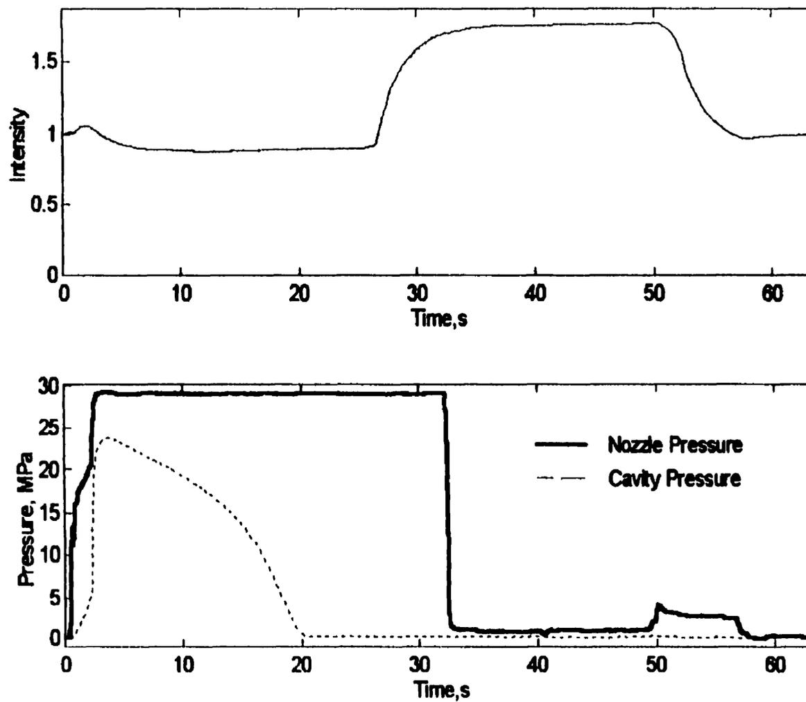
**Figure 4.5A Plots of reflection intensity and pressure for polystyrene, low pressure experiment - PS/LP**
