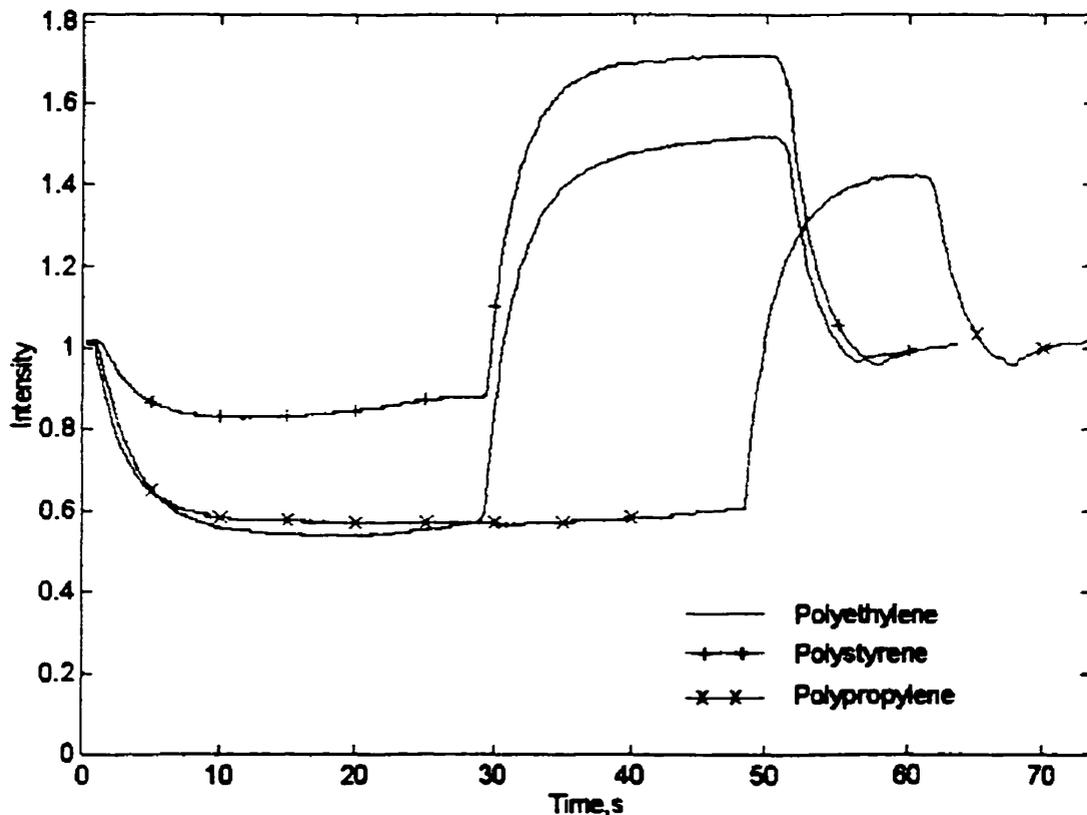
Figure 4.2 Comparison of reflection intensities for polyethylene, polypropylene, and polystyrene.
