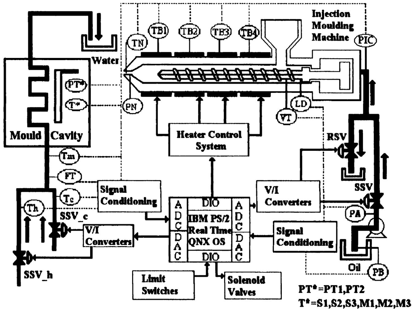
Figure 3.1 Instrumentation of the McGill Injection Moulding Machine.
