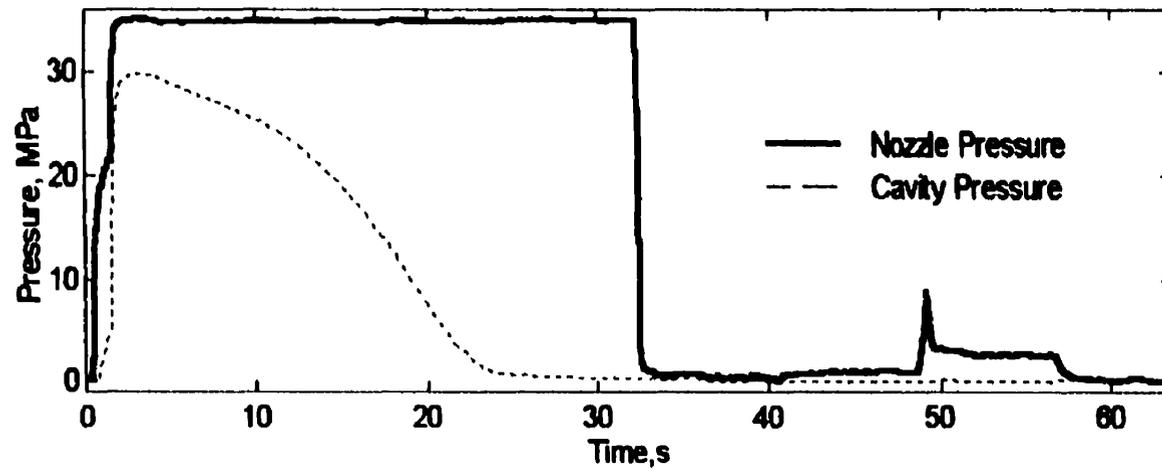
**Figure 4.8B** Plots of reflection intensity and pressure for polystyrene, high cooling temperature experiment - PS/HT
