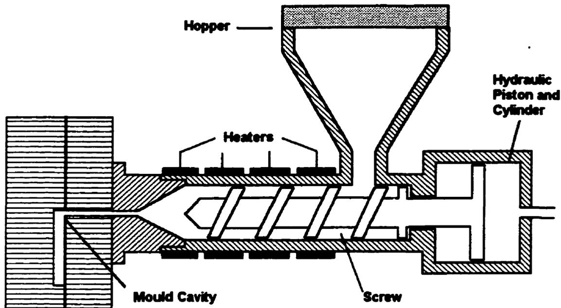
**Figure 2.1 Sketch of a reciprocating injection moulding machine**
