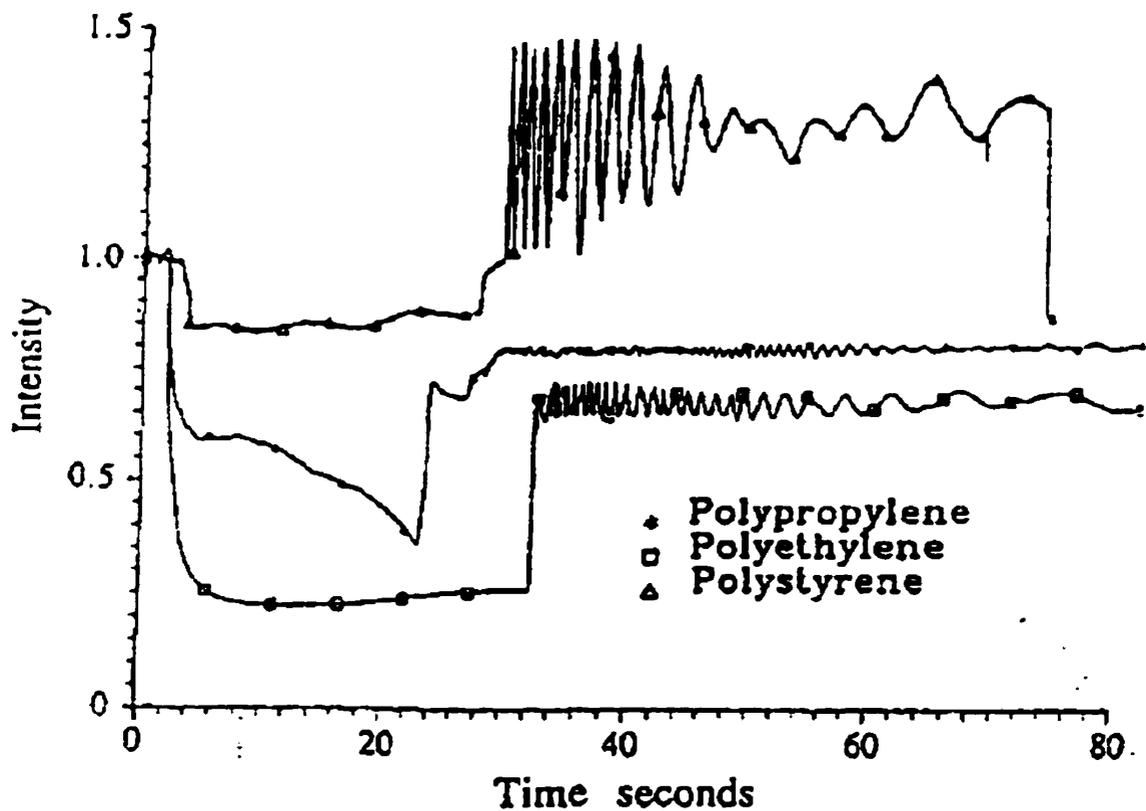
**Figure 4.9 Reflection intensity curves obtained by Bur and Thomas [12].**
