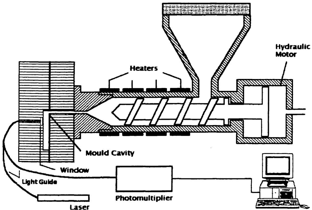
**Figure 3.4 Optical sensing apparatus installed on the injection moulding machine**
