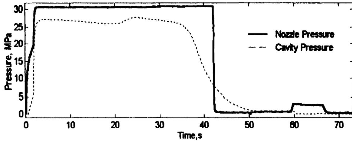
**Figure 4.4A** Plots of reflection intensity and pressure for polypropylene, low pressure experiment - PP/LP
