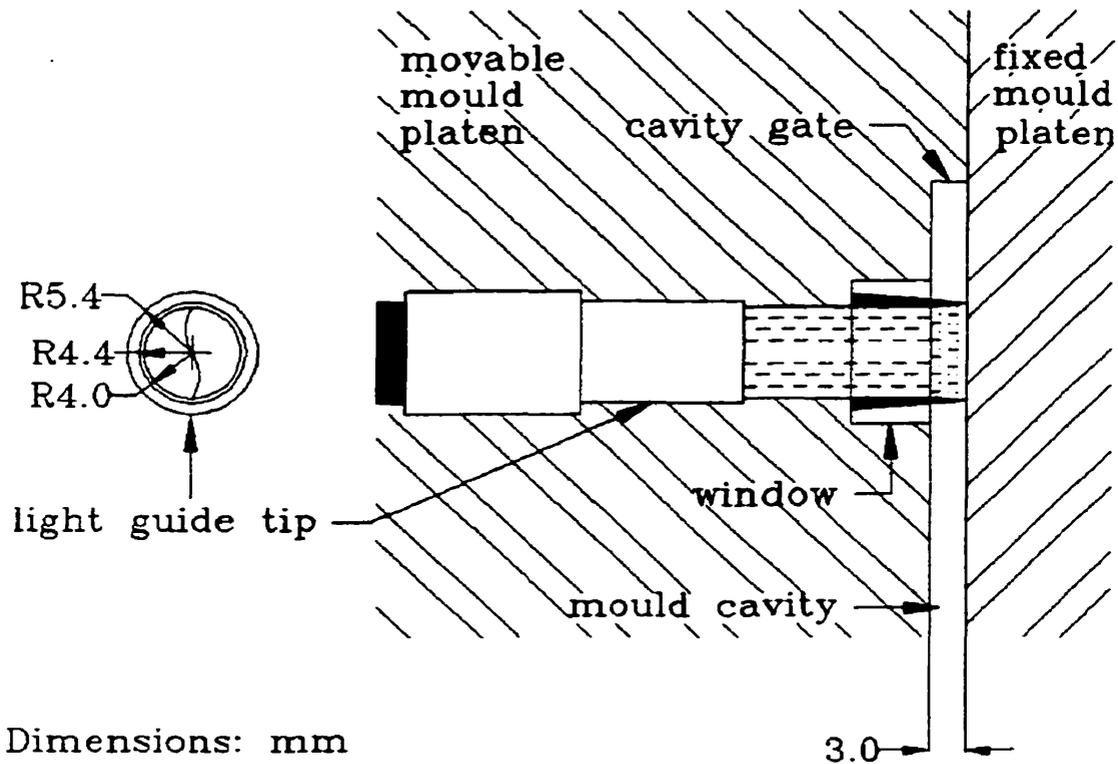
**Figure 3.2 Installation of light guide and window on the movable mould platen. R4.0 corresponds to the fiber bundle radius (inner circle); R4.4 is the radius of a metal bundle sheath (middle circle), and R5.4 is the radius of a metal ferrule (external circle).**
