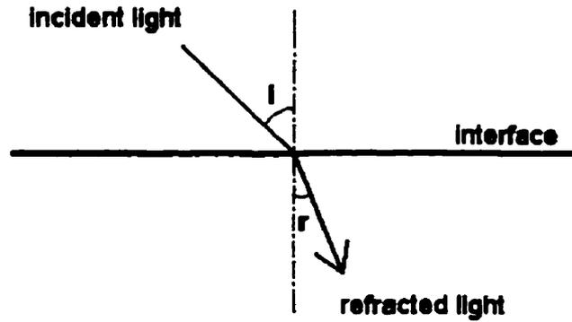
**Figure 2.4 Refraction of light**
