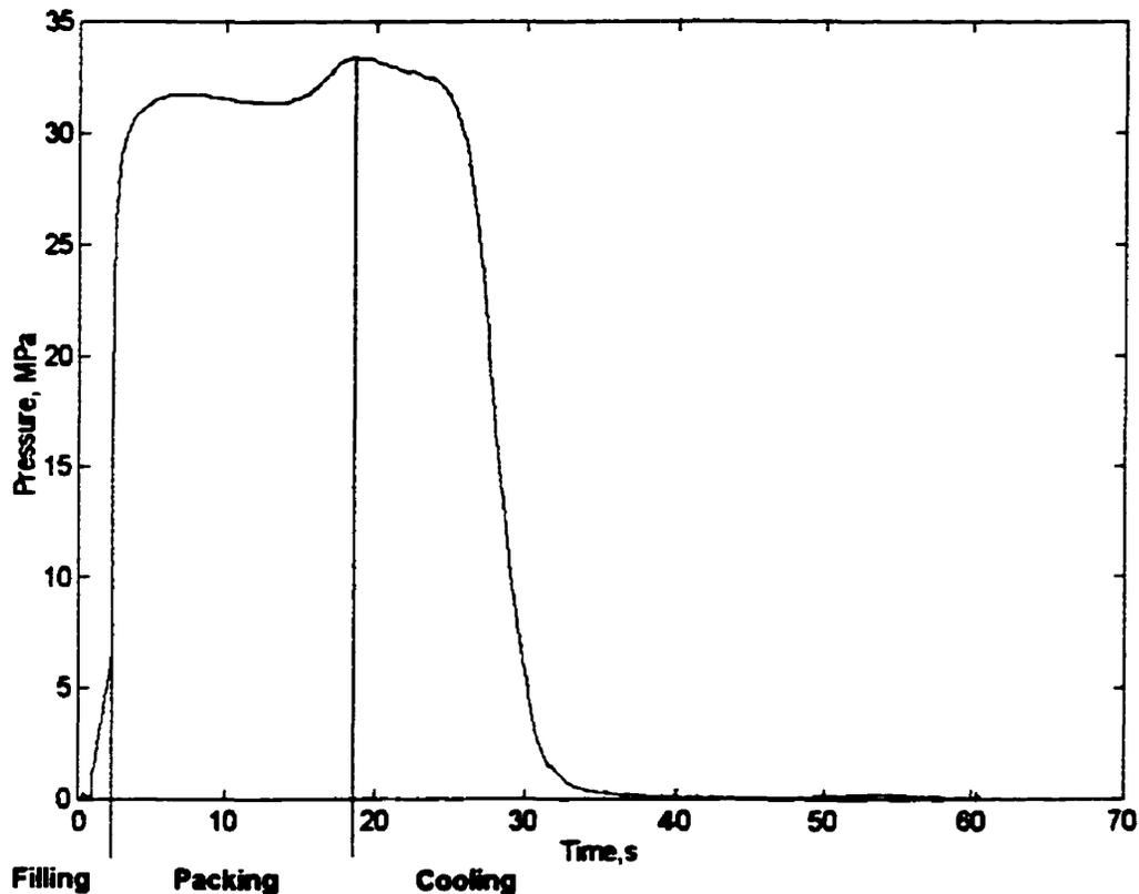
**Figure 2.2 Typical profile of cavity pressure during an injection moulding cycle for HDPE**
