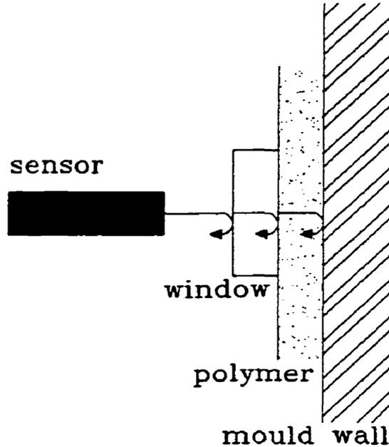
**Figure 2.3 Configuration of the optical sensor proposed in [12]**
