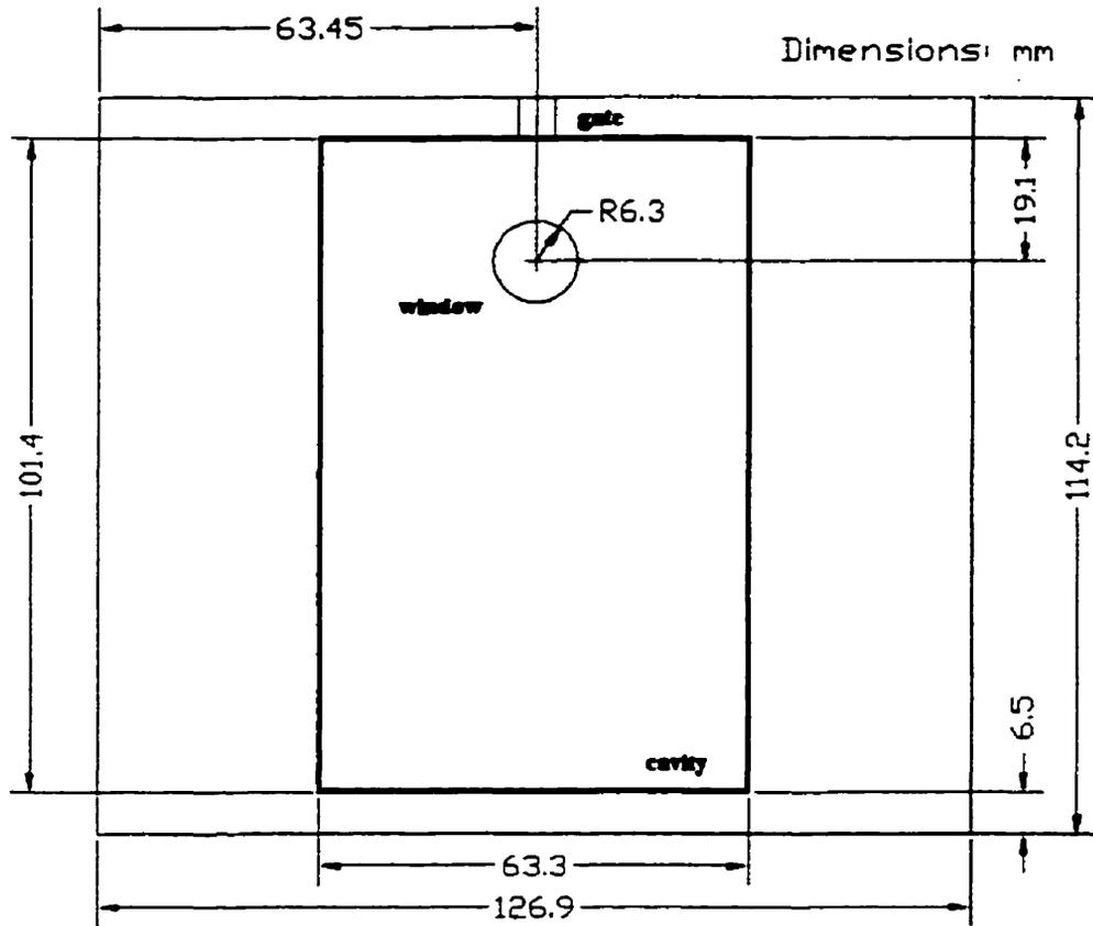
**Figure 3.3 Position of the window on the mould insert**
