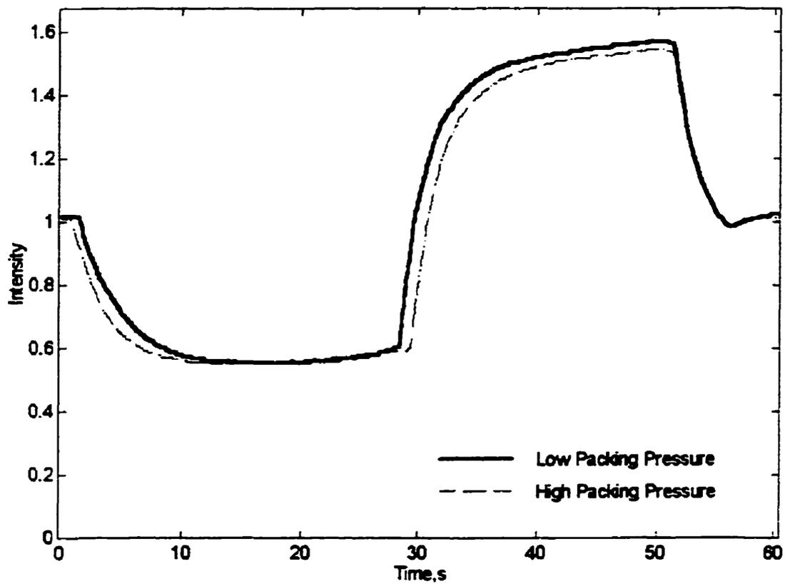
**Figure 4.3C Comparison of intensities from the HDPE/LP and HDPE/HP experiments**
