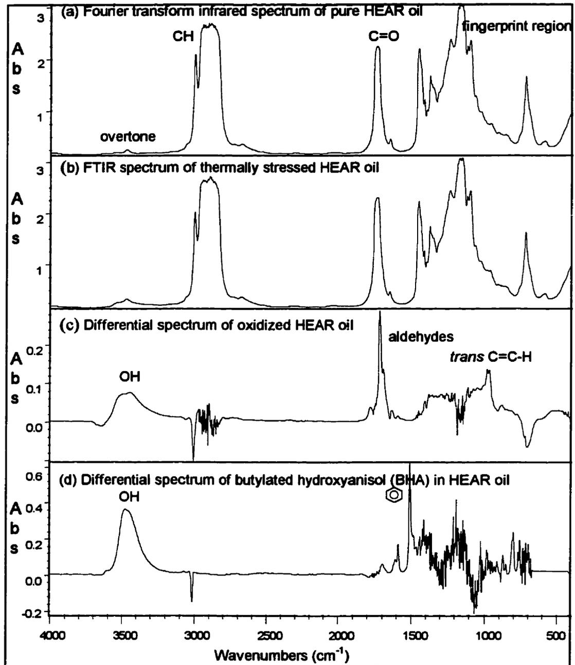
Figure 16. (a) Fourier transform infrared spectrum of pure HEAR oil; (b) pure HEAR oil heated at 100°C with dry air bubbled through @ ~3ml/min for 48 hours; (c) the differential spectrum obtained by ratioing b against a; and (d) differential spectrum obtained by ratioing the HEAR oil spiked with 1% (w.t.) BHA against that of the pure HEAR oil
