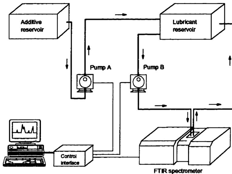
**Figure 14. A schematic diagram of the COAT System and flow pattern**
