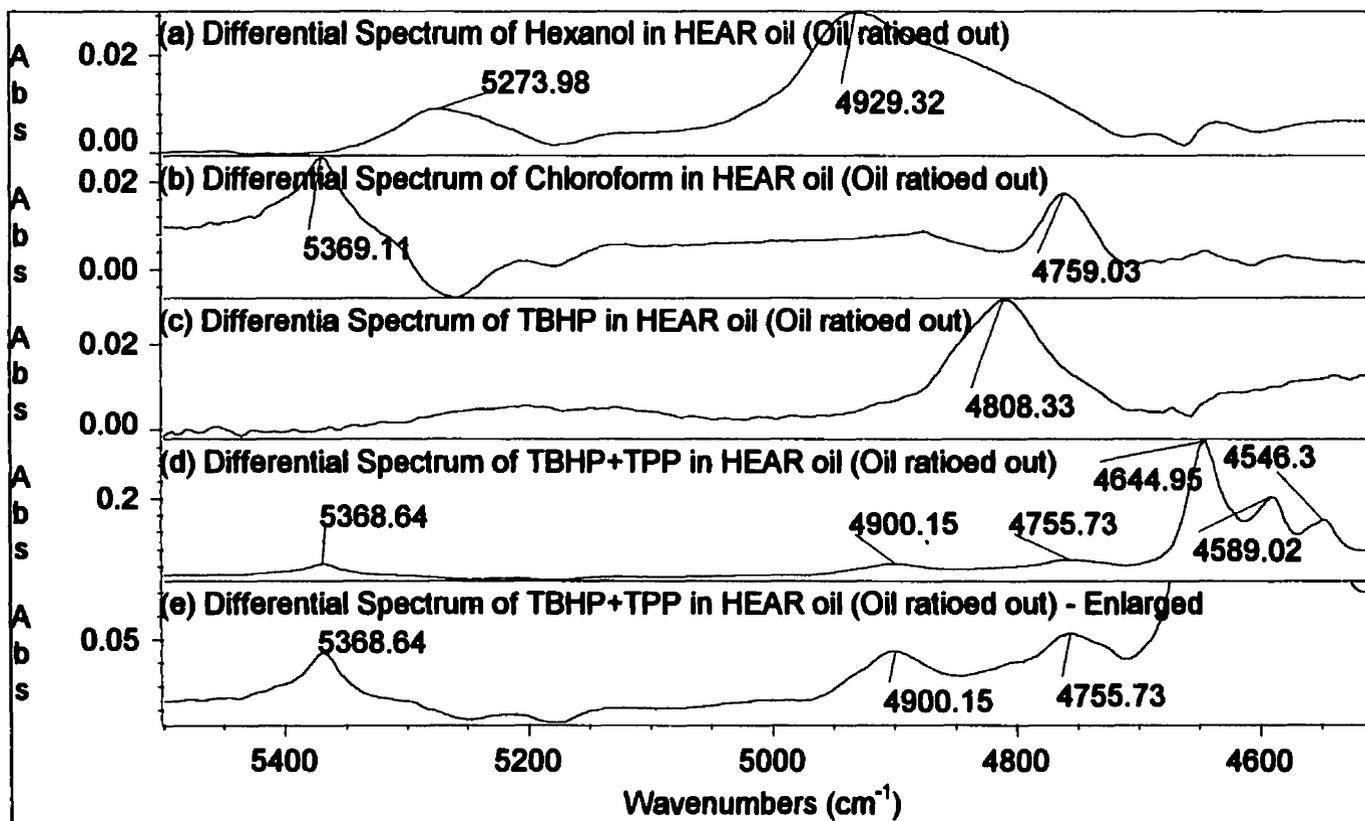
Figure 8. Differential spectra of hexanol, chloroform, TBHP and reacted TBHP and TPP in HEAR oil after ratioing out the HEAR oil spectral contributions.
