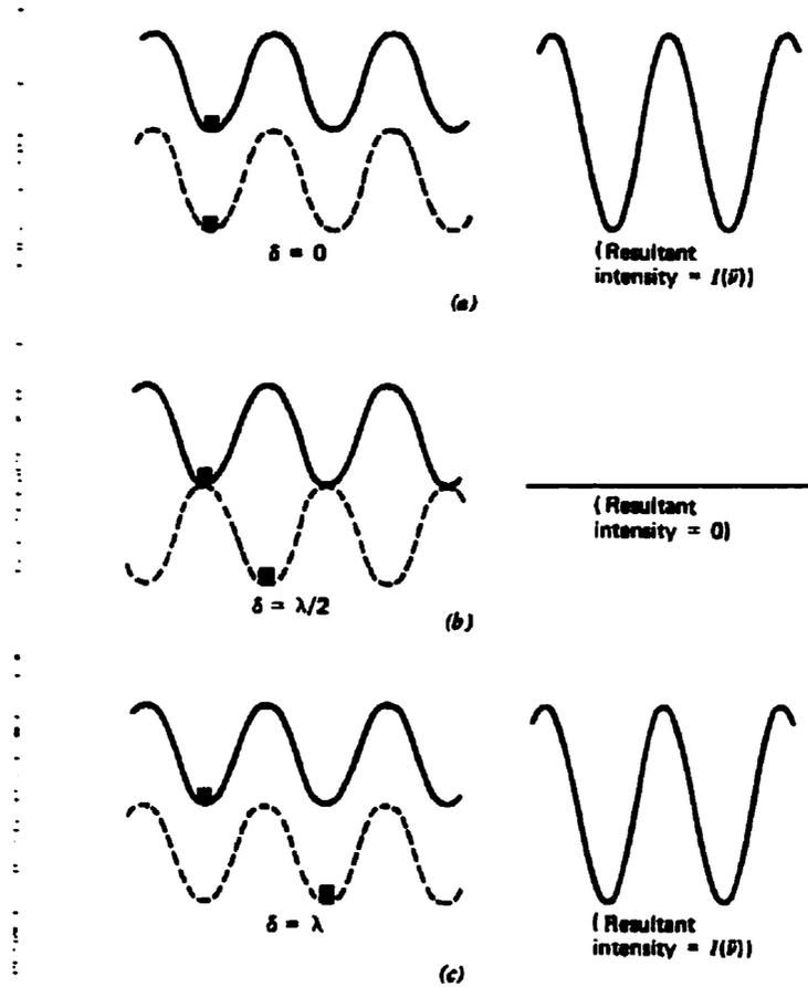
Fig 5. Schematic diagram of the phase of the electromagnetic waves from the fixed mirror (solid line ) and movable mirror (broken line) at different values of the optical retardation. (a) Zero path difference; (b) path difference of one-half wavelength; (c) path difference of one wavelength. (Griffiths and Hasethk, 1986)
