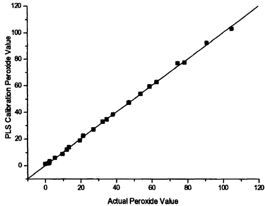
**Figure 10. Plot of the predicted peroxide value vs. the actual peroxide value for the 23 calibration standards as derived from the partial least squares calibration (PLS)**
