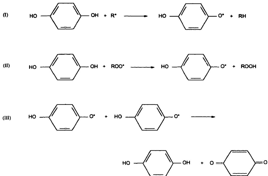
Figure 3. The mechanism for the antioxidation reaction of hydroquinone
