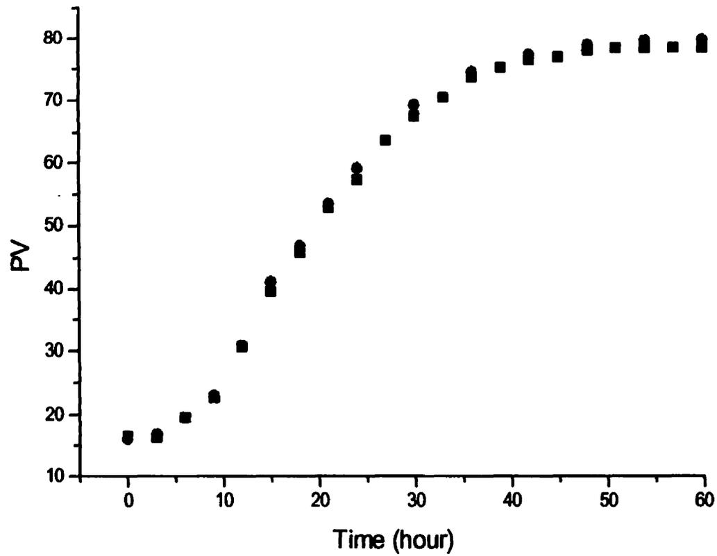
**Fig 13. Real-time AOM plot of HEAR oil under forced thermal/oxidation conditions comparing FT-NIR (■) and iodometric (●) PV results**
