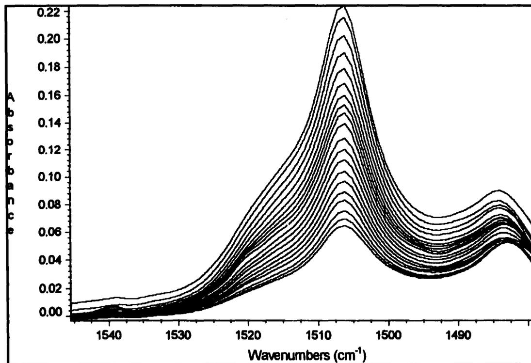
Figure 17. Spectral overlay plot illustrating changes at 1508 cm<sup>-1</sup> of 0.5% (w.t) TBHQ spiked in HEAR oil heated at 100°C and bubbled with dry air @ ~ 3ml/min as a function of time. The overlaid spectra were collected at 3 hour intervals and have been ratioed against the spectrum of the clean HEAR oil.
