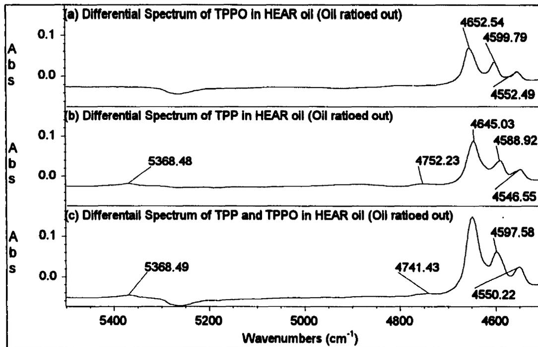
Figure 7. Differential spectra of TPP, TPPO, and a 1:1 TPP/TPPO mixture in HEAR oil after ratioing out the HEAR oil spectral contribution
