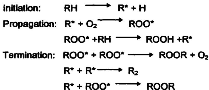
Figure 1 Primary steps in autoxidation reaction (Paquette, et al., 1985a)
