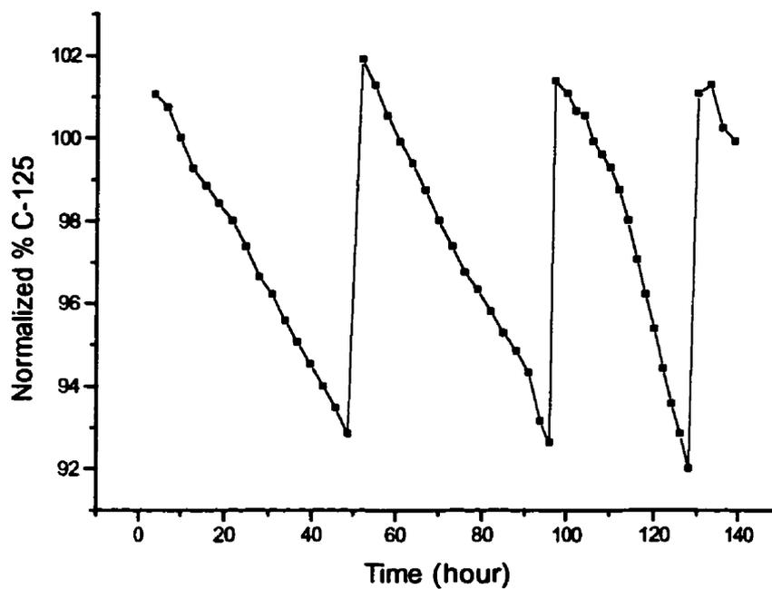
Figure 19. Real-time replenishment plot of C-125 added in mineral base oil heated at 100°C with dry air bubbled through @ ~3 ml/min.
