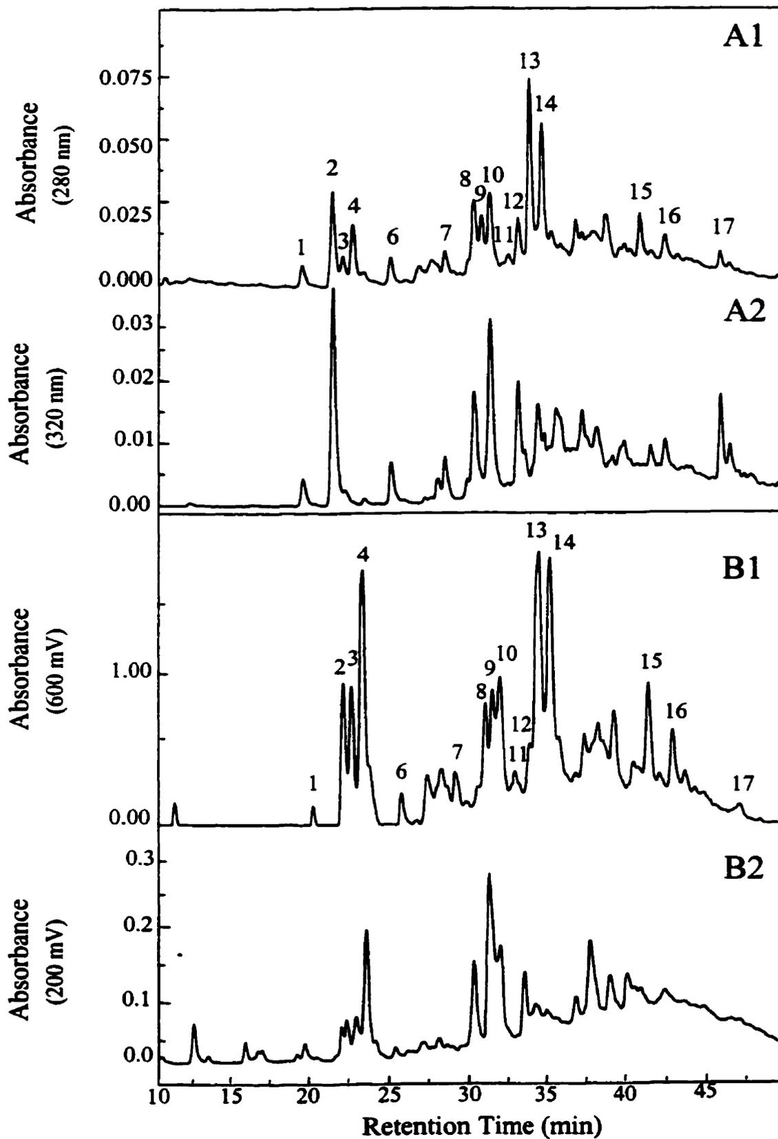
Figure 14. Chromatograms of HPLC analysis of phenolic compounds and flavonoids obtained from maple syrup at 0% of the season using UV diode-array detector at 280nm (A1) and 320 nm (A2) as well as electrochemical (EC) detector at 200 mV (B2) and 600 mV (B1).
