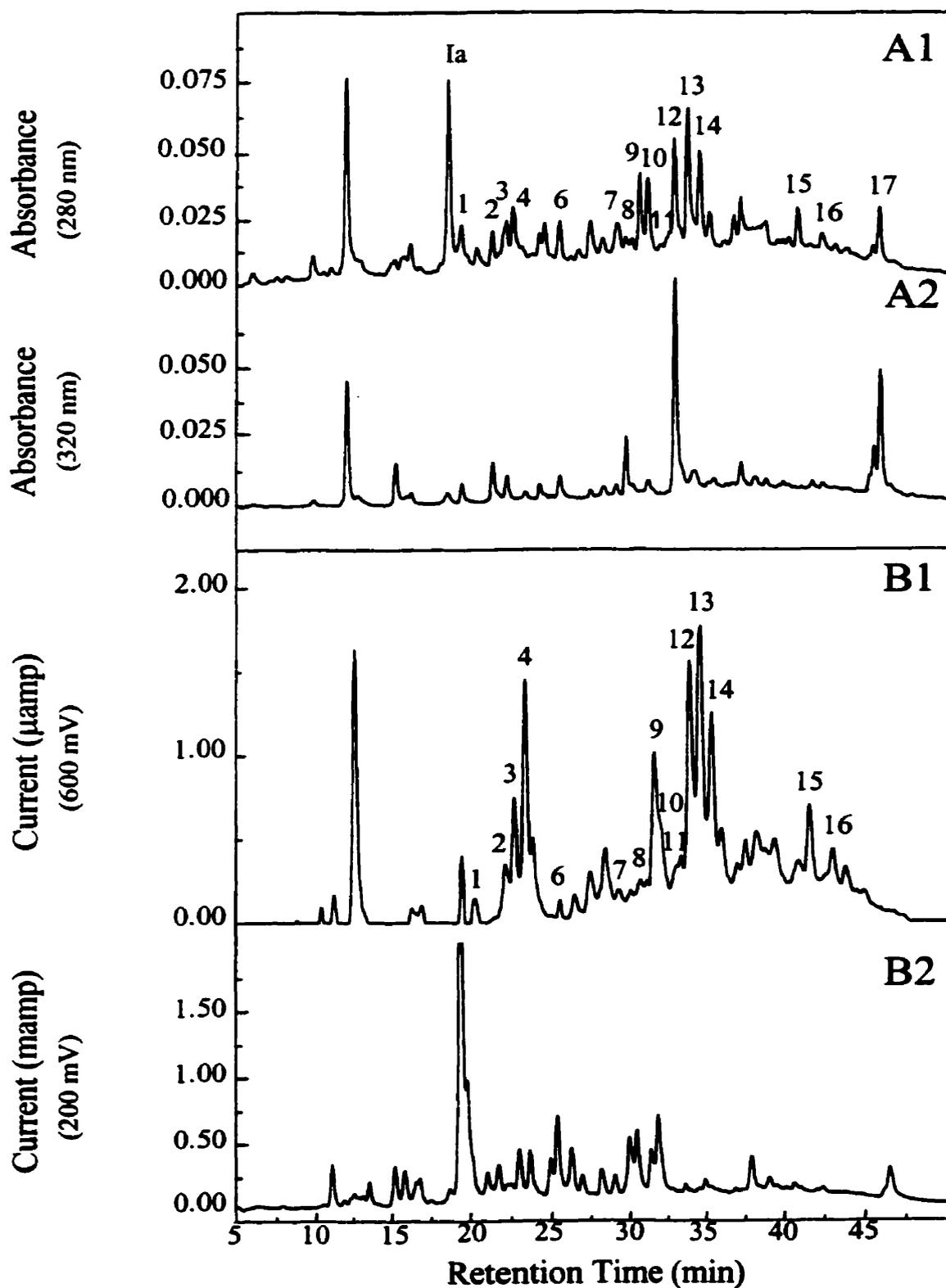
Figure 15. Chromatograms of HPLC analysis of phenolic compounds and flavonoids obtained from maple syrup at 100% of the season using UV diode-array detector at 280 nm (A1) and 320 nm (A2) as well as electrochemical (EC) detector at 200mV (B2) and 600 mV (B1).
