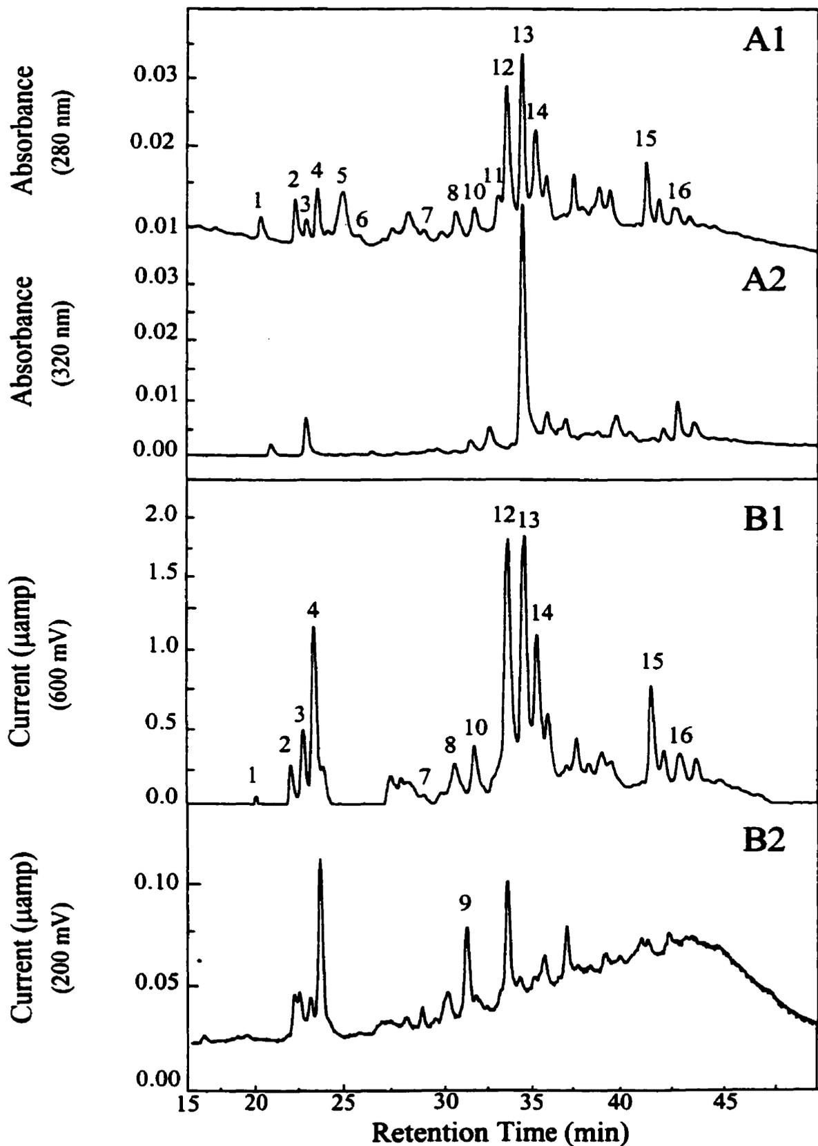
Figure 9. Chromatograms of HPLC analysis of phenolic compounds and flavonoids obtained from maple sap at 100% of the season, using UV diode-array detector at 280 nm (A1) and 320 nm (A2) as well as electrochemical (EC) detector at 200 mV (B2) and 600 mV (B1).
