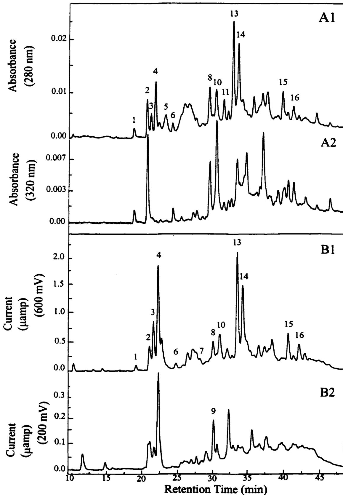
Figure 8. Chromatograms of HPLC analysis of phenolic compounds and flavonoids obtained from maple sap at 0% of the season, using UV diode-array detector at 280 nm (A1) and 320 nm (A2) as well as electrochemical (EC) detector at 200 mV (B2) and 600 mV (B1).
