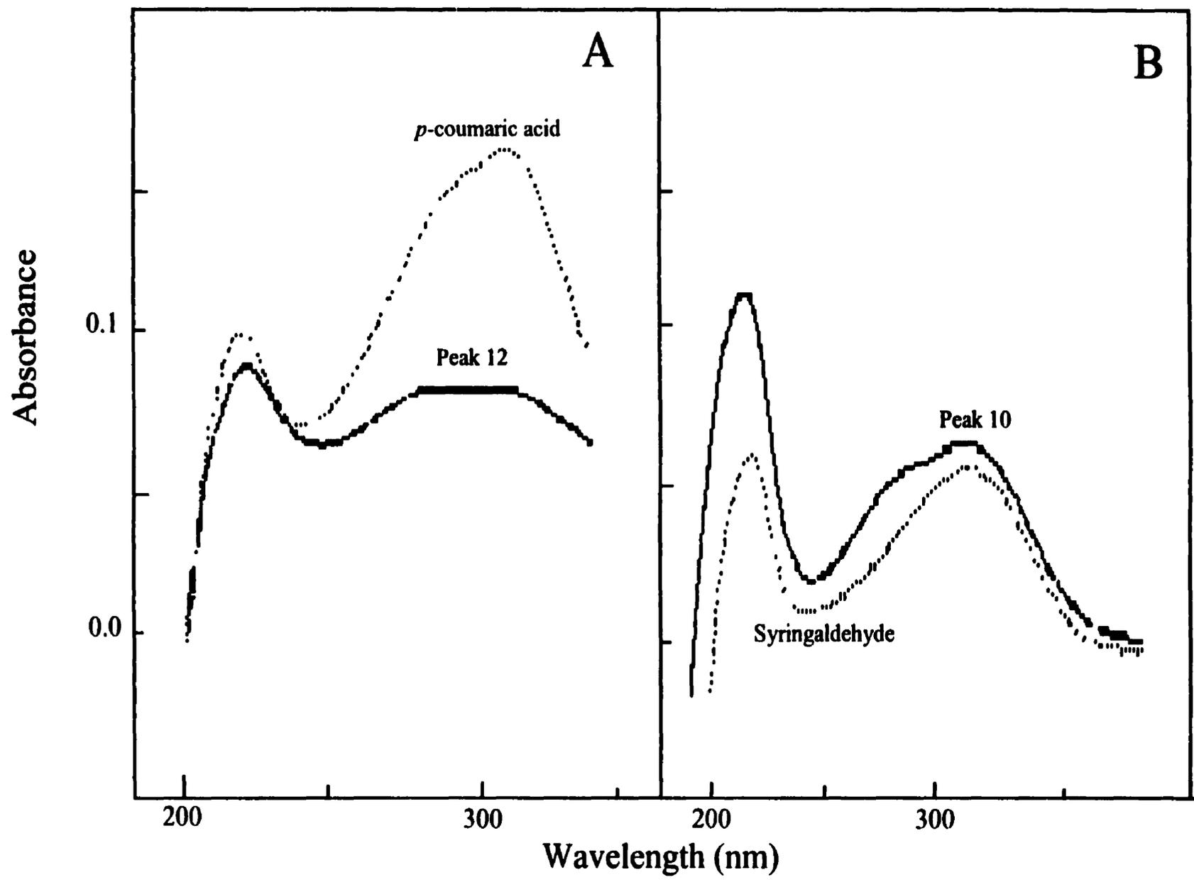
Figure 11. Scan spectrum comparison of standard phenolic compounds and identified peaks from figure 8, 9, 14 and 15 obtained from maple sap and maple syrup at different periods of the season. (A) *p*-coumaric acid and peak 12, (B) syringaldehyde and peak 10.
