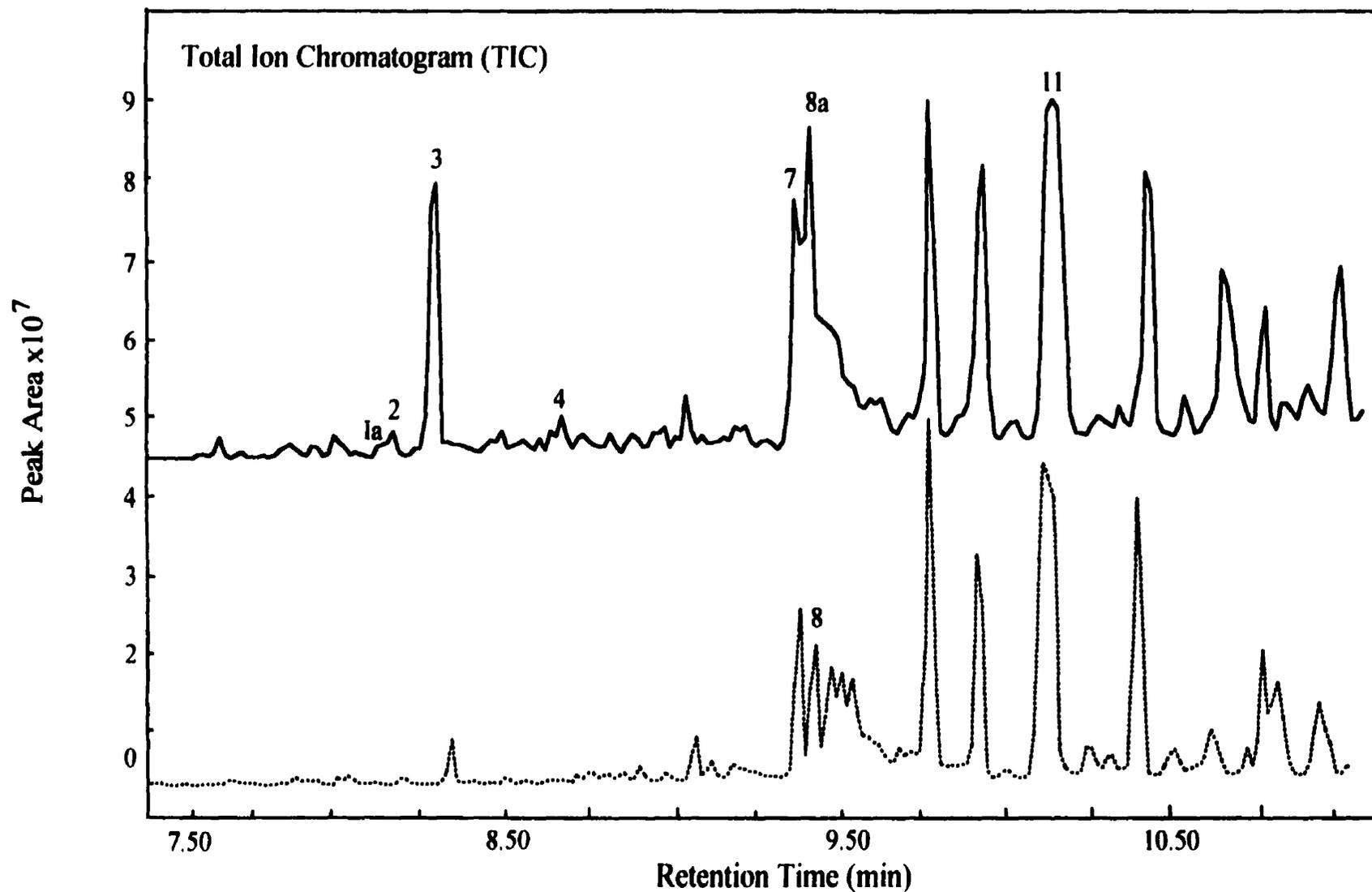
Figure 17. GC/MS analysis of phenolic compounds and flavonoids obtained from maple sap (.....) and maple syrup (—) at 100% of the season. Including, vanillin (1a), 1, 2, 3-trioxybenzene (2), 3-hydroxy-capric acid (3), syringaldehyde (4), protocatechuic acid (8a) and coniferol / *p*-coumaric acids (11) from Table 12.
