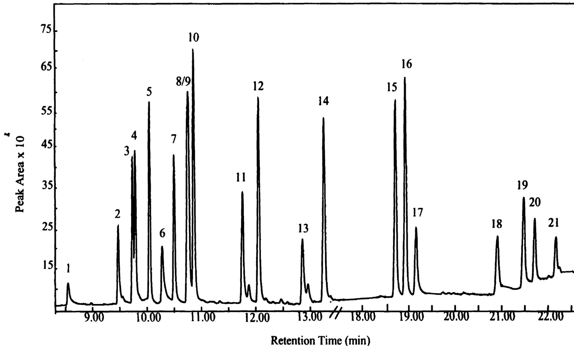
Figure 5. Chromatogram of GC analysis of phenolic and flavonoid standards including, vanillin (1), syringaldehyde (2), vanillic acid (3), homovanillic acid (4), protocatechuic acid (5), coniferal (6), syringic acid (7), coniferol (8), *p*-coumaric acid (9), gallic acid (10), ferulic acid (11), caffeic acid (12), sinapic acid (13), *trans*-resveratrol (14), (-)-epicatechin (15), (+)-catechin (16) hesperetin (17), kaempferol (18), fisetin (19), chlorogenic acid (20) and quercetin (21).
