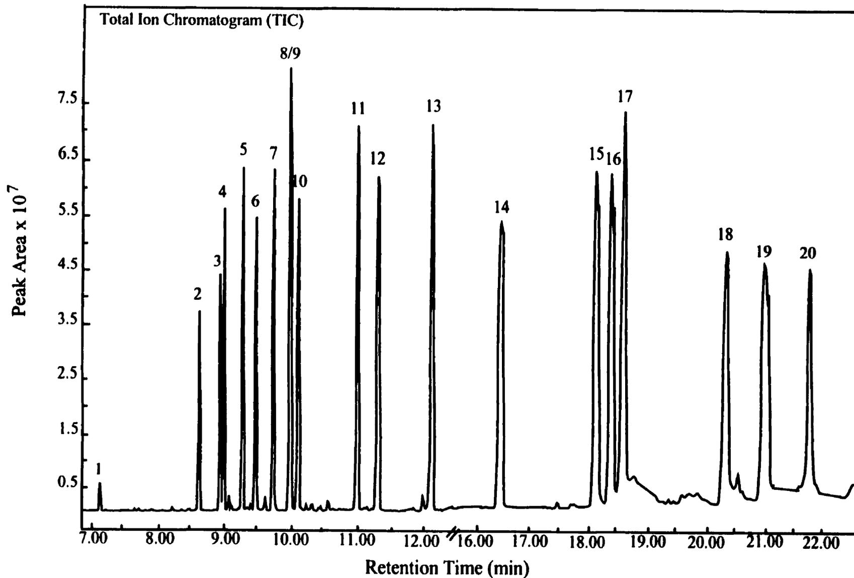
Figure 7. GC/MS analysis of phenolic compounds and flavonoid standards including, vanillin (1), syringaldehyde (2), vanillic acid (3), homovanillic acid (4), protocatechuic acid (5), coniferal (6), syringic acid (7), coniferol (8), *p*-coumaric acid (9), gallic acid (10), ferulic acid (11), caffeic acid (12), sinapic acid (13), *trans*-resveratrol (14), (-)-epicatechin (15), (+)-catechin (16), hesperetin (17), kaempferol (18), fisetin (19), chlorogenic acid (20).
