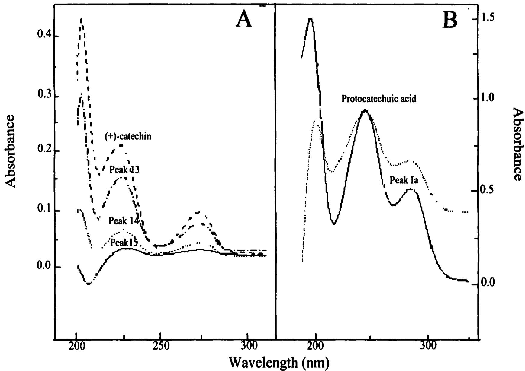
Figure 12. Scan spectrum comparison of phenolic and flavonoid standards and identified peaks from figure 8, 9, 14 and 15 from maple sap and maple syrup at different periods of the season. (A) (+)-catechin and flavanol related compounds, peak 13, 14 and 15. (B) protocatechuic acid and peak 1a identified in maple syrup only starting at 50% of the season.
