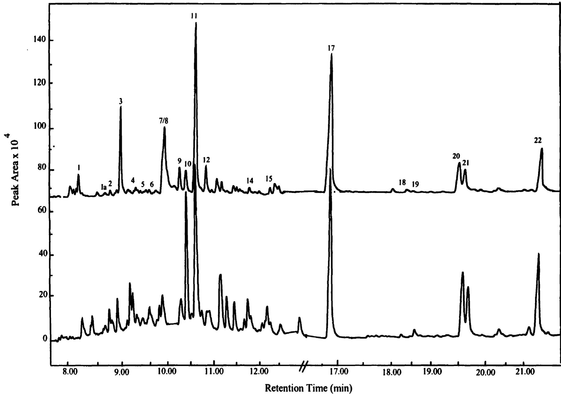
Figure 16. Chromatograms of GC analysis of phenolic compounds and flavonoids obtained from maple syrup at 0% (lower line) and 100% (upper line) of the season using flame ionization detector (FID).
