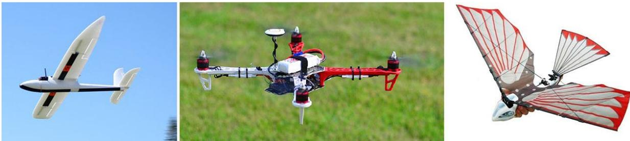
Figure 1.1: Examples of fixed-wing (left), rotary-wing (center), and flapping-wing (right) UAVs.
