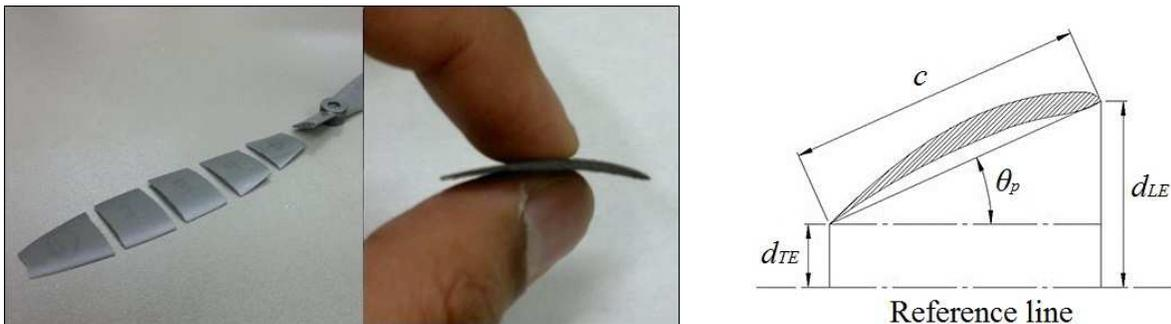
Figure 4.12: Segmented Electrify 10x4.5 propeller.
