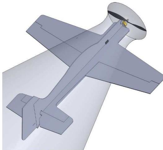
Figure 5.1: Propeller slipstream on a small fixed-wing UAV.
