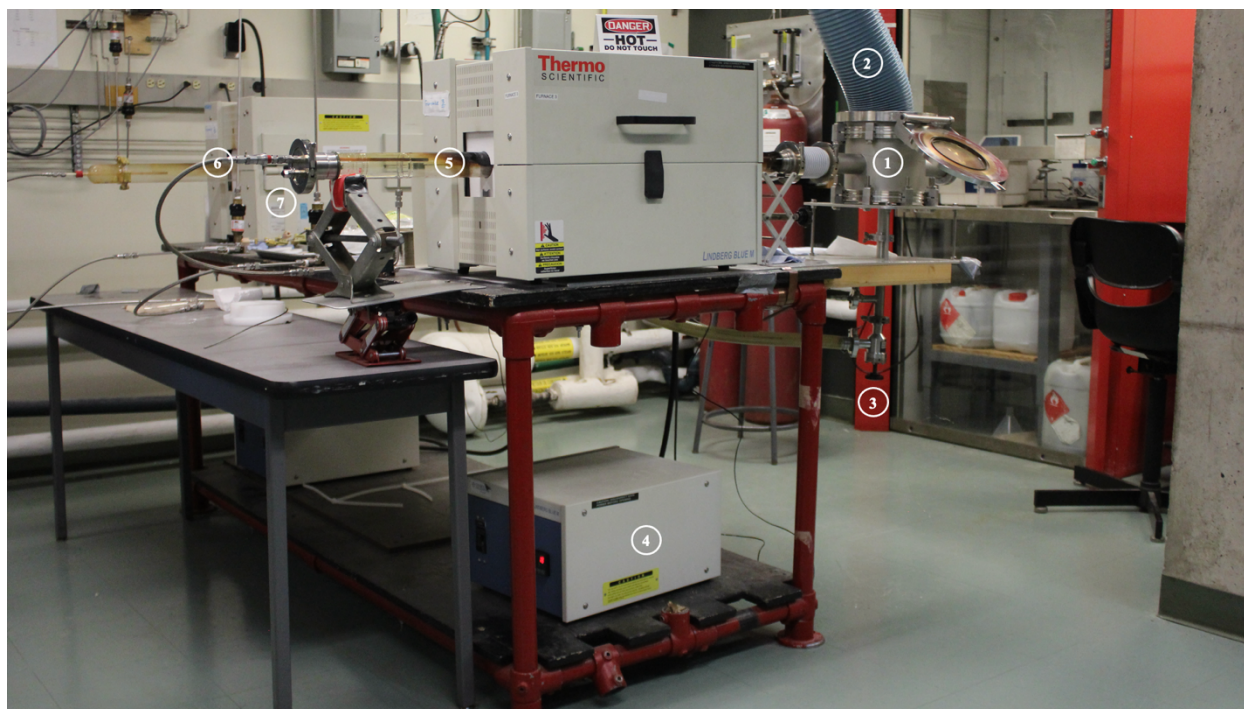
Figure 10: Side view of the t-CVD setup in the CPPE laboratory (1) Loading chamber (2) Elephant trunk hose (3) Gas exhaust valve (4) Furnace control panel (5) Furnace tube (6) Gas flow inlet (7) Wire to pull Quartz boat
