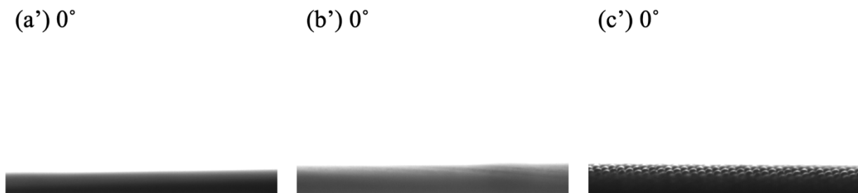
Figure 33: WCAs of MWCNT and NH 2 -MWCNT filters (a-a') 5 \mu m (b-b') 10 \mu m (c-c') 25 \mu m
