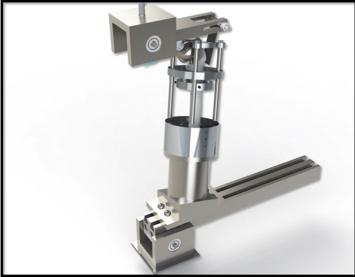
Figure 28: Physiological loading jig that simulates stair climbing with attached micromotion fixture to measure the movement at the bone implant interface.
