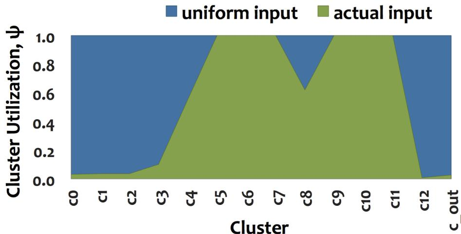
**Fig. 3.2** Clusters utilization comparison of uniform (randomly generated) and real (actual network trace) inputs.
