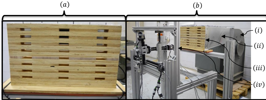
Figure 6-2: (a): Front view of the static model ducts, (b): View of the static model showing the blower (i), HVAC duct (ii), static model ducts (iii), and the motorized axes (iv)
