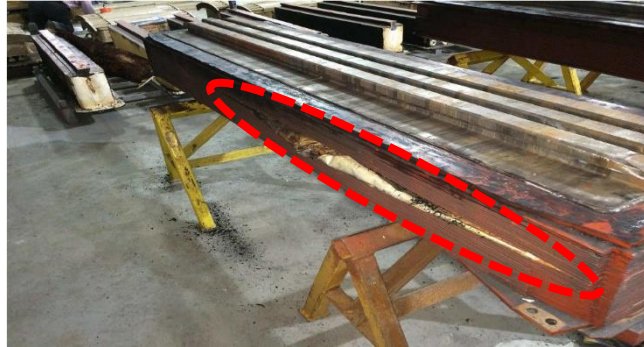
Figure 1-4: Burnt rotor pole
