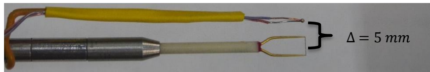
Figure 6-3: Hot-wire/thermocouple combination used for simultaneous multi-point measurements
