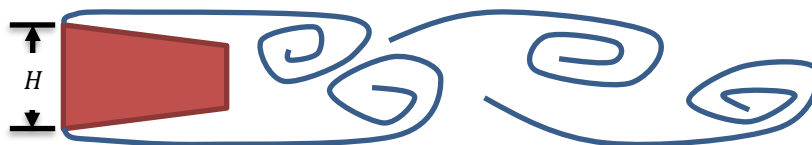
Figure 4-5: Sketch of a vortex flow meter (top view)
