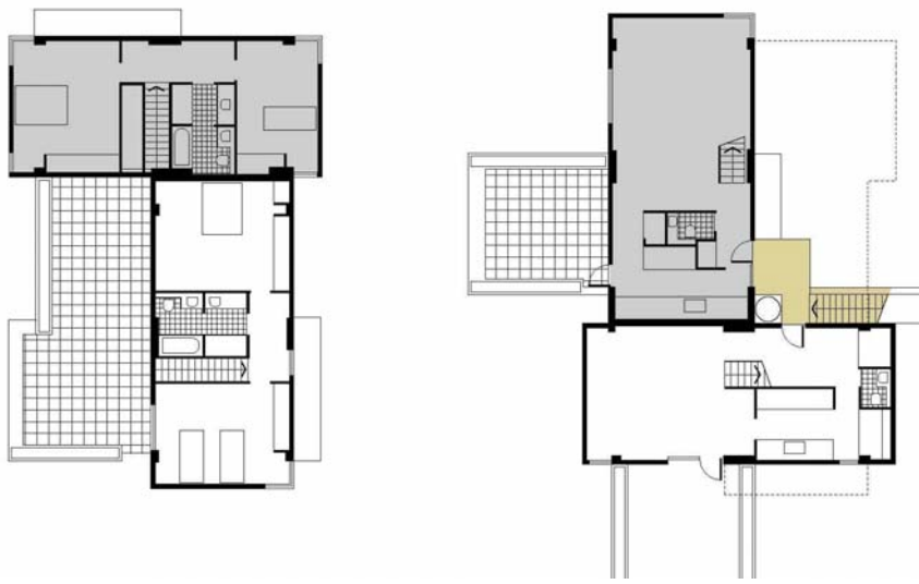
Figure 3.3.6-3.3.8: Modular units forming a variety of house plans
