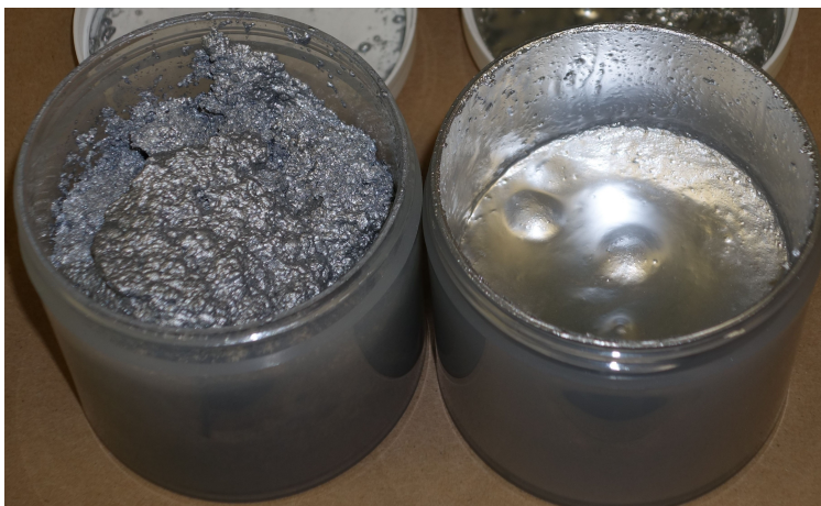
Figure 3.7: Flake-Al mixture before (left) and after (right) acoustic mixing.
