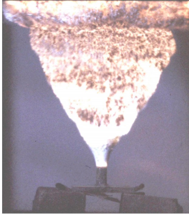
Figure 2.2: Detonation propagation through a long tube of aluminized NM explosive from Haskins et al. [3].
