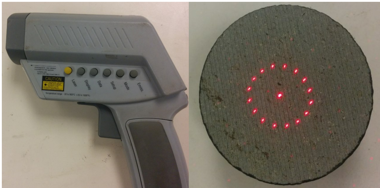
Figure 3-3. The infrared thermometer (left) area on basalt disk over which temperature is averaged (right)
