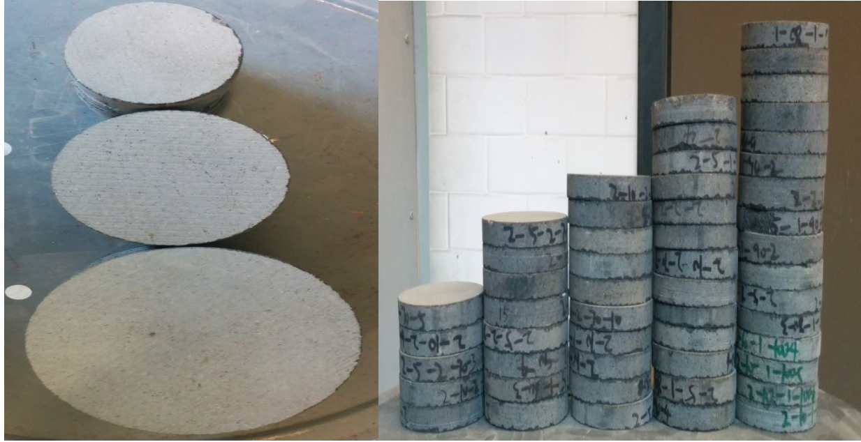
Figure 3-6. Cylindrical cores were grouped by three diameters (left), and for each diameter, disks were stacked to form 5, 8, 10, 13 and 16 cm cylinders (right)
