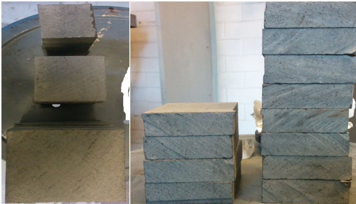
Figure 3-7. Cubic disks were grouped by side length (left) and for each side length the disks were stacked to form 10 and 16cm cores (right)
