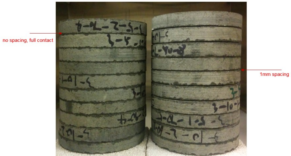
Figure 3-8. Two 10-layer cores without (left) and with (right) 1mm air spacing between each layer
