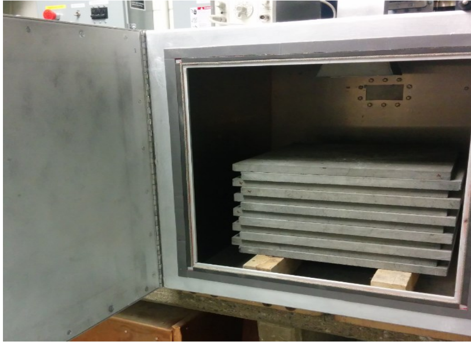
Figure 2-19. A multimode cavity with conducting walls and horn antenna connecting to a waveguide
