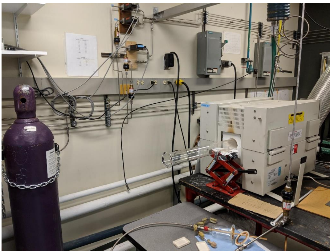
Figure 13: Tube furnace serving as the pyrolysis reactor used in the PPL lab.
