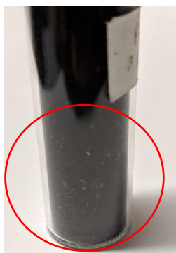
Figure 19: Platinum agglomeration in catalyst sample marked with red circle.
