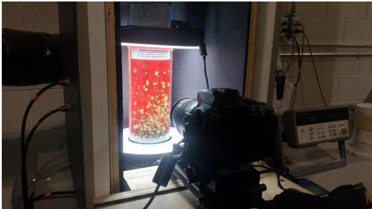
Figure 4.8 Component of the real-time image acquisition system for fluidized bed drying [26]
