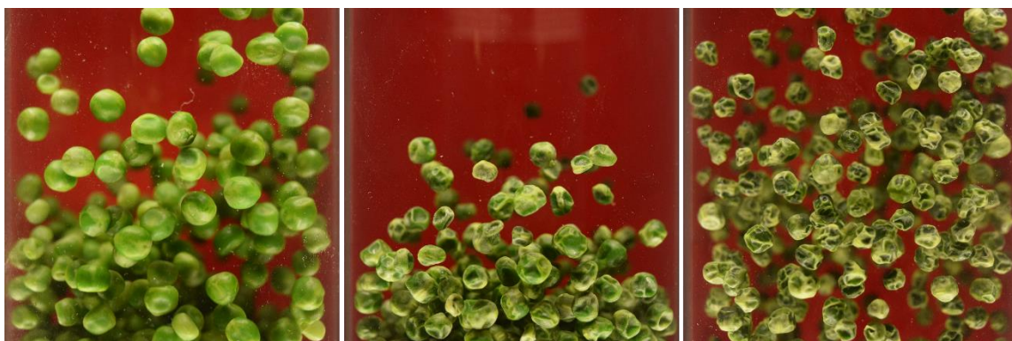
Figure 4.2 Images of green peas captured during fluidized bed drying [26]
