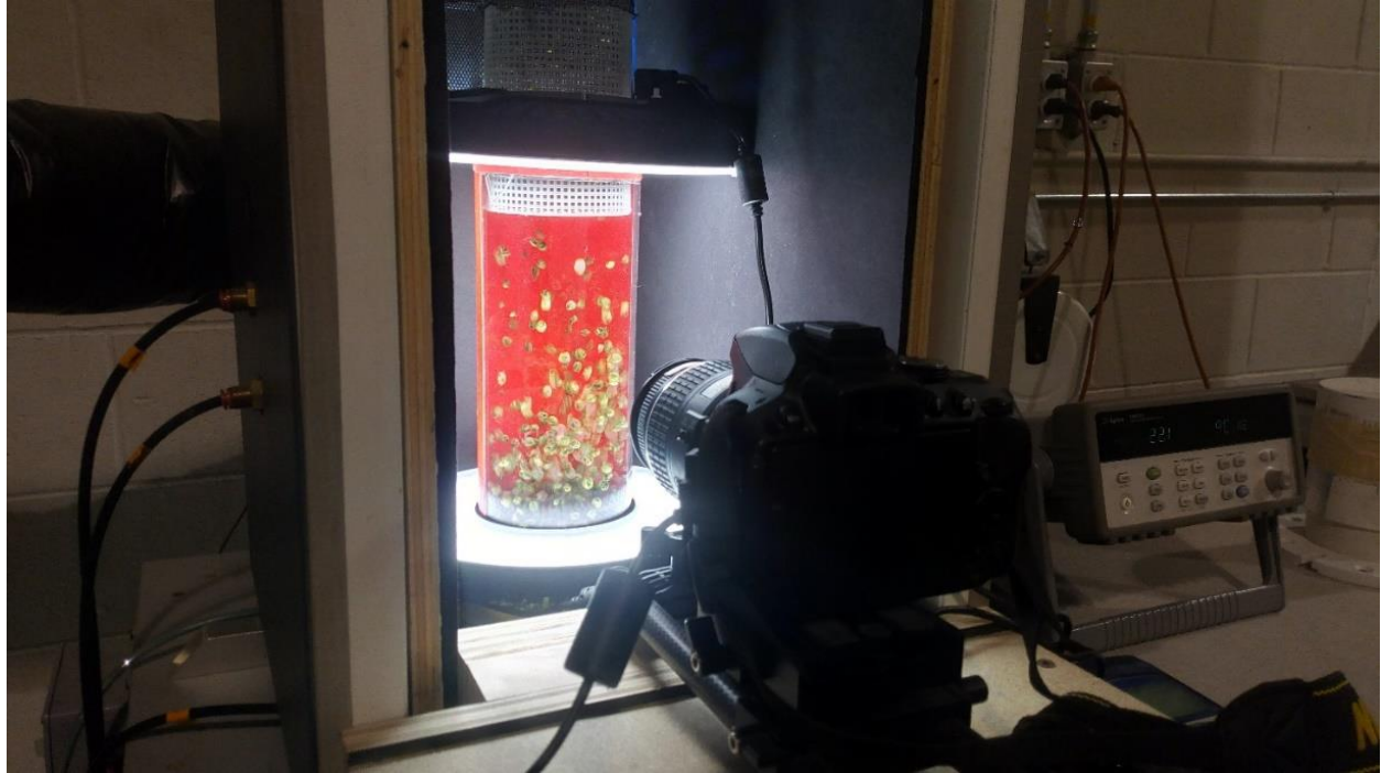
Figure 3.3 Component of the real-time image acquisition system for fluidized bed drying
