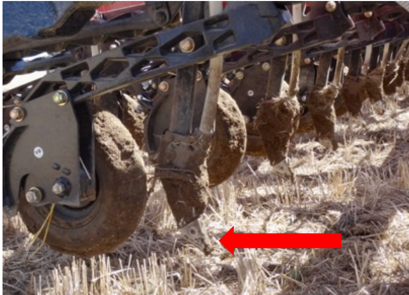
Figure 29. The Narrow Knife Opener. The two-inch wide knife openers on the red hoe drill seeding implement with packer wheels behind. The red arrow is pointing to one of the knife openers. Photo by Katherine Strand
