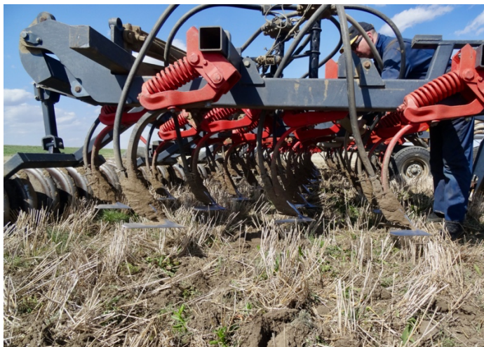
Figure 22. Organic Seeding. Pictured above is a seeding implement in use by an organic farmer. The V-shaped blades are mounted in front of the seed opener and designed to disturb weeds while seeding. Photo by Katherine Strand.
