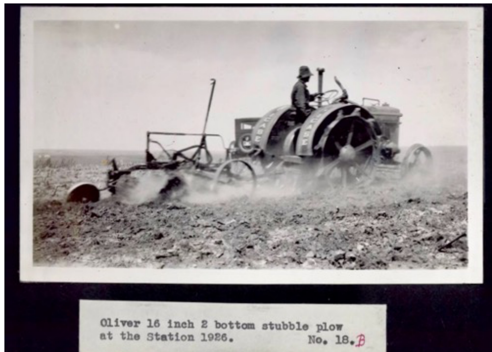
Figure 33. Pre-working the Field. A laborer from the Station driving an open air tractor and pulling a mouldboard plough to pre-work a field prior to seeding. Note the original caption. Photo from SCRDC Archives
