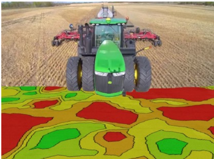
Figure 67. Variable Rate Field Zones. The above shows typical field zone (polygon) map, superimposed on a photo of a farmer seeding. Photo from Center Field Solutions Ltd (2020).
