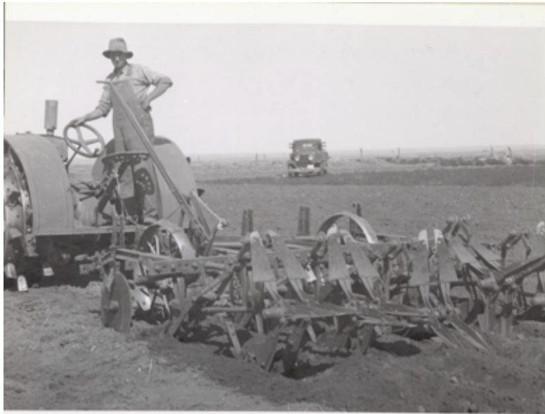
Fig. 1 - Rear view of machine in operation. Center dammer shown completing a dam. Second dammer from right in act of tripping.
