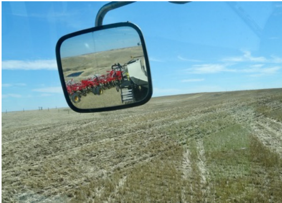
Figure 32. John's View from the Cab. The view from inside the tractor cab with the rearview mirror reflecting the hoe drill implement. Notice the faint line between the perfectly erect stubble on the right and the slightly flattened stubble on the left. The left side has been seeded.
