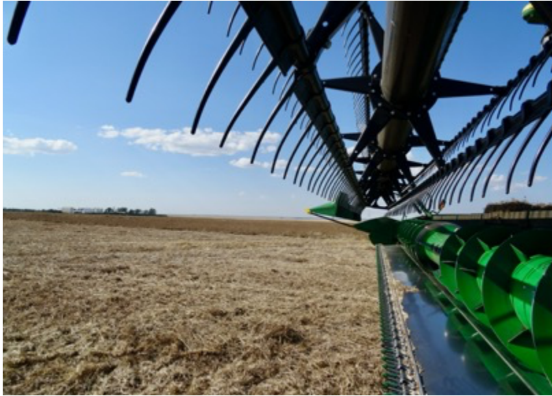
Figure 3. The Header. Pictured above is an example of a combine header with the cutting blade at the bottom, spinning reel towards the top, and auger in the center. Photo by Katherine Strand.
