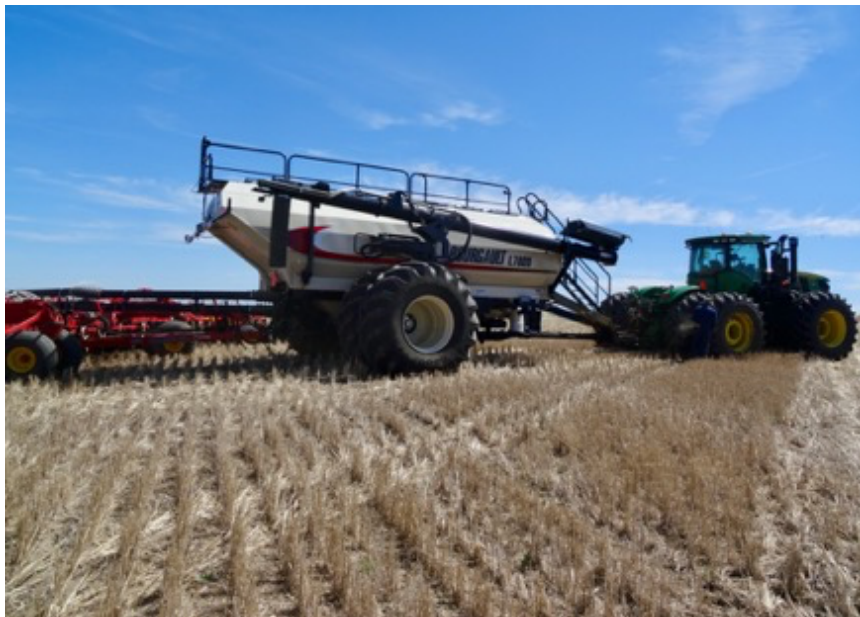
Figure 27. John's New Bourgault. The zero tillage seeding equipment with the tractor hitched to the white air seeder cart, which is hitched to the red hoe drill seeding implement. Notice the erect crop stubble on the field. Photo by Katherine Strand.
