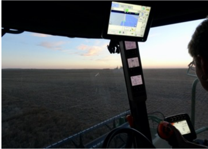
Figure 7. Autodrive. Pictured above is Hannah H. and the computer interface in her combine—note the joystick in the lower right corner and the GPS screen in the upper part of the photo. Photo by Katherine Strand.
