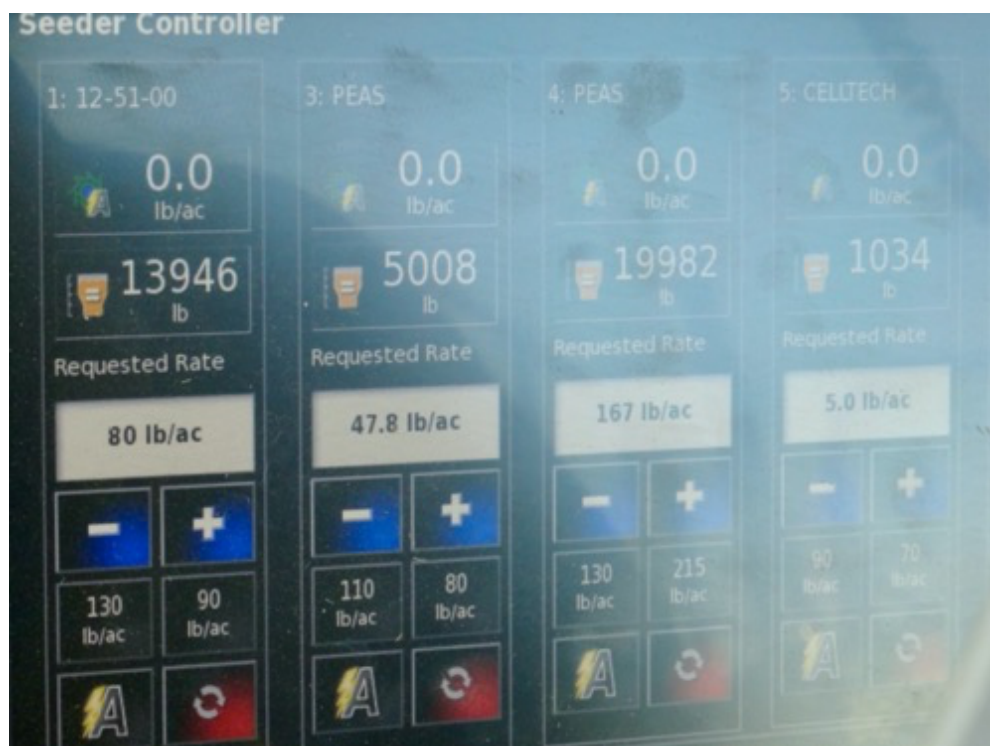
Figure 66. Seed and Fertilizer. This photo shows the in-cab computer interface that farmers use to set their rates of seed and fertilizer as pounds/acre. Photo by Katherine Strand
