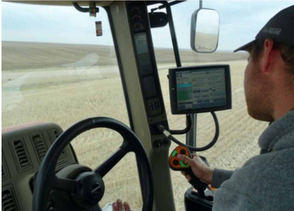
Figure 58. Derek in the Patriot. The photo shows the sprayer cab with controls and the computer GPS interface. Photo by Katherine Strand.
