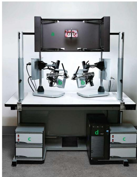
Figure 1 NeuroTouch simulator components: a) stereoscope/ visual feedback, b) haptic systems, c) power supplies and amplifiers for haptic systems, d) high-performance computer
