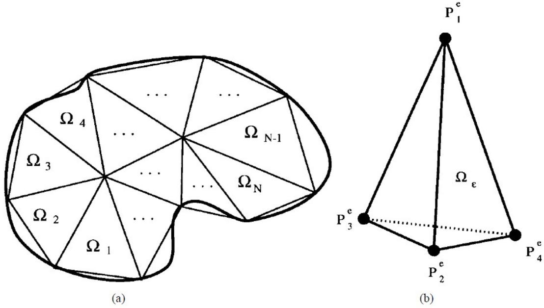
Figure 4 FEM example: left: Discretization of the domain into finite elements (2D illustration), right: the volumetric mesh consists with tetrahedral finite elements.
