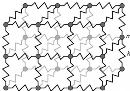
Figure 3 Mass-spring system: each circle contributes a mass point and links by structural springs which are controlled by stiffness.
