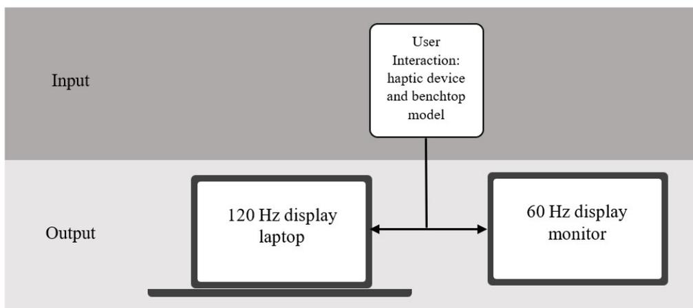
Figure 1 The platform set-up. Left is the laptop that runs the 120Hz display, the haptic device and benchtop model are in the middle, and right is the external touch-screen running the 60Hz display. The surgeon operates the haptic device based on the visual feedback from both monitors
