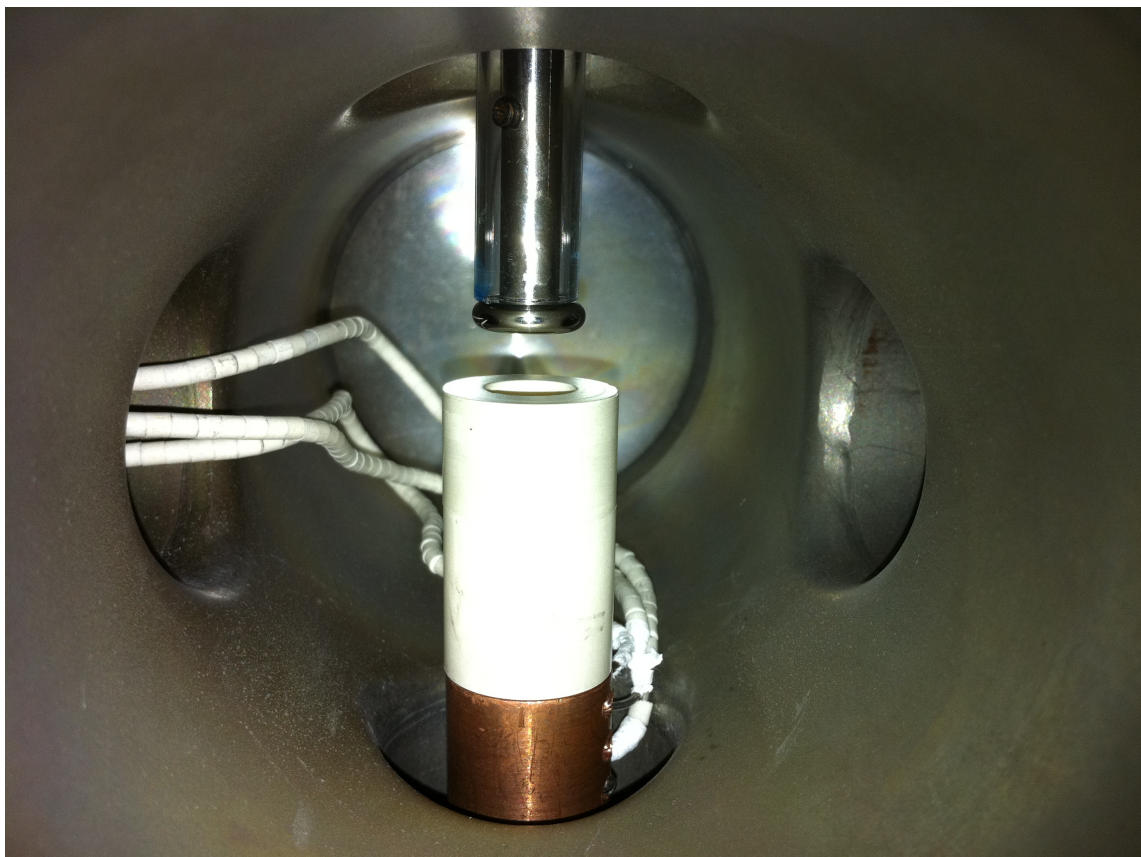
Figure 3-4: A photo of the interior of the DC glow discharge chamber, depicting the BN cathode holder, Al anode (top), the inner borosilicate glass tube, and water-cooled cathode (bottom). Note that in this photo, the outer borosilicate glass tube has been removed.
