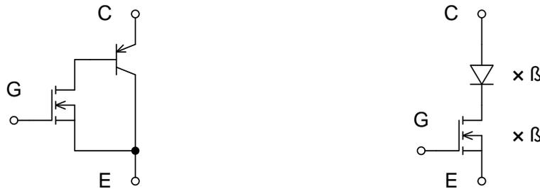
Figure 3-2: IGBT DC models: basic (left), simplified (right)
