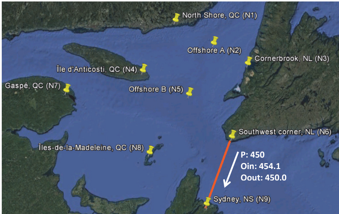
Figure 10 – Power flow in MW, Case 2 (P: Planning; O: Operations) – background map: Retrieved from Google Earth [42]
