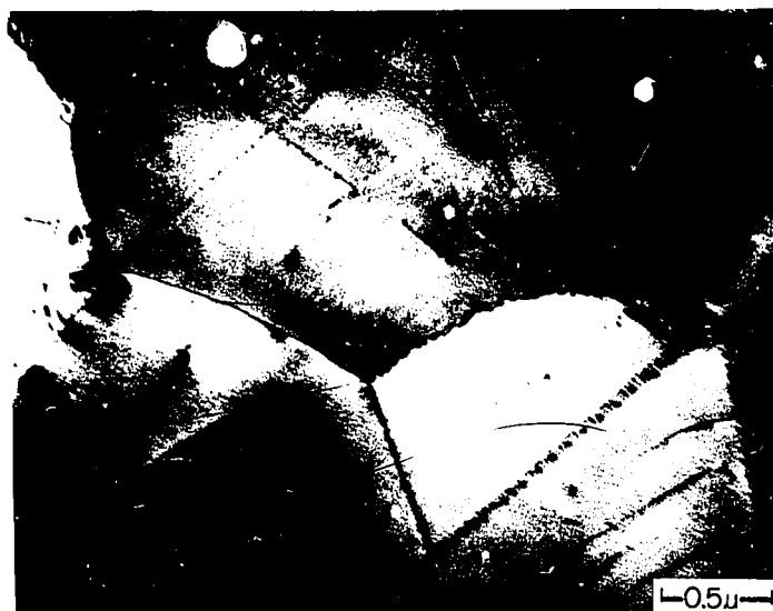
Fig. 86 - Silicon steel; 800°C; \epsilon = 0.76 ; \dot{\epsilon} = 0.15/\text{sec} ; delay 40 sec; TEM; 28,600 X.
