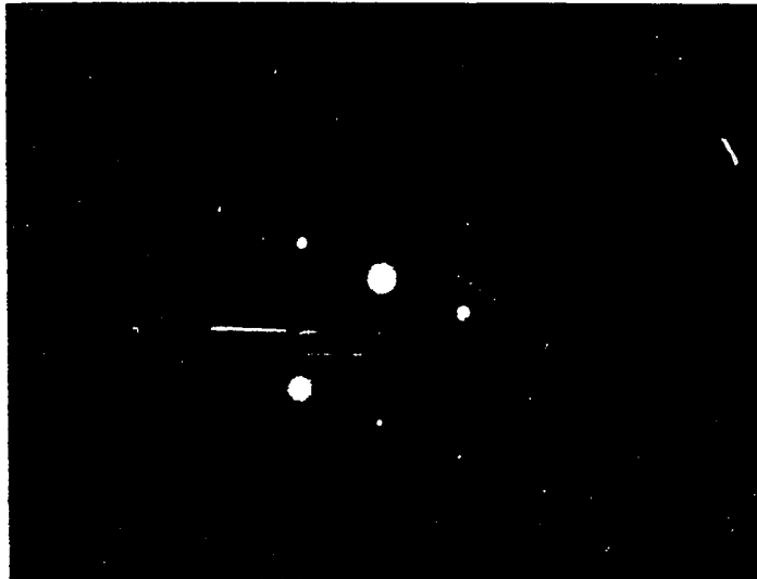
Fig. 8 - Superimposed transmission electron diffraction patterns of 2 adjacent subgrains. Armco iron; 600°C; \xi = 0.56 .
