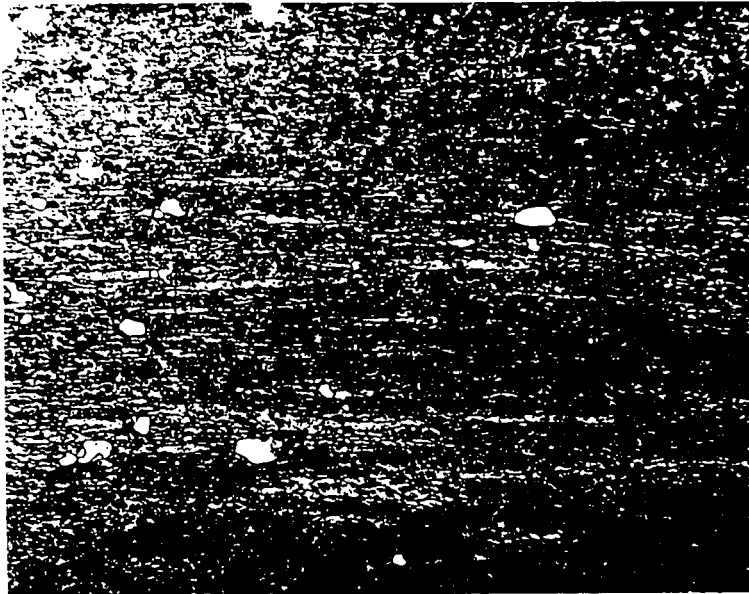
Fig. 52 - Silicon steel; 560°C; \varepsilon = 1.67 ; \dot{\varepsilon} = 0.42/\text{sec} ; delay 20 min; EPE; 220 X.
