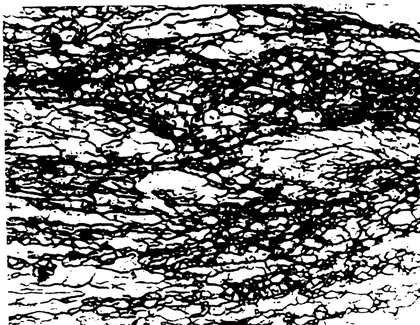
Fig. 58 - Silicon steel; 650°C; \epsilon = 1.32 ; \dot{\epsilon} = 0.25/\text{sec} ; delay 5 sec; EPE; 680 X.
