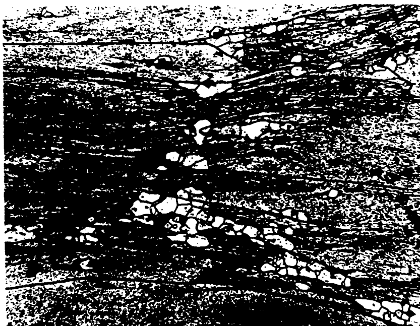
Fig. 89 - Silicon steel; 560°C; \epsilon = 1.67 ; \dot{\epsilon} = 0.42/\text{sec} ; delay 25 min; EPE; 220 X.
