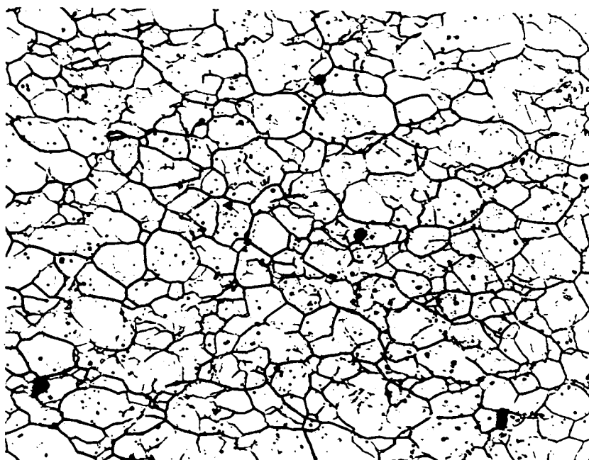
Fig. 69 - Silicon steel; 1,000°C; \epsilon = 0.53 ; \dot{\epsilon} = 0.08/\text{sec} ; delay 1 sec; EPE; 220 X.
