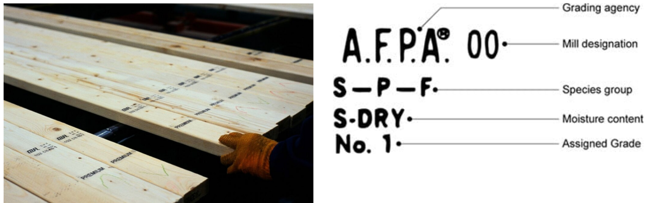
Figure 13 – Visual grader inspecting dimensional lumber (left) and Example lumber grade stamp (Source: Canadian Wood Council 2021). (Photo: "Naturally:Wood | British Columbia's Sustainable Forestry Resource," n.d.)
