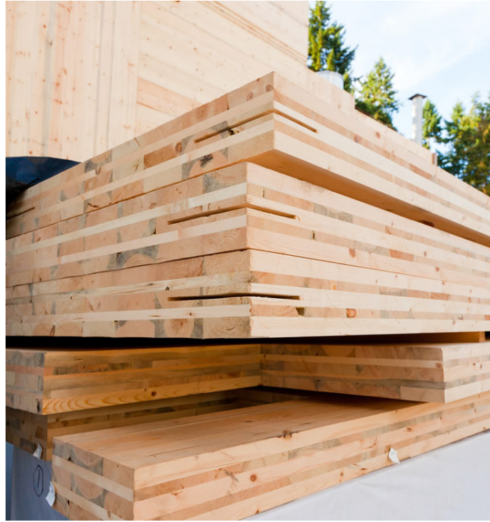
Figure 21 - CLT panels waiting for installation. (Photo: N. R. Canada 2014)
