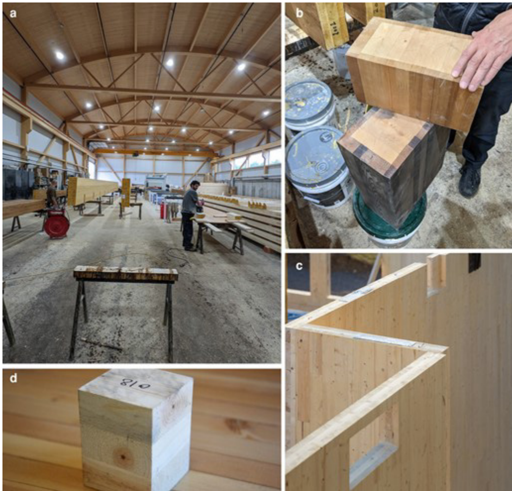
Figure 29 - a) Mass timber manufacturing facility near the study region (Art Massif, Saint-Jean-Port-Joli, Quebec) and b) test samples of a mixed hardwood veneer and glulam beam (photos: Osborne et al. (48)). c) Sample of a custom CLT panel utilizing low-value ponderosa pine (Muszynski et al. 2022) . Popular industry CLT panel manufactured with black spruce (90% by volume) and other common building species (spruce, pine, and fir; typically known as SPF). Reproduced from Osborne et al. (2023).
