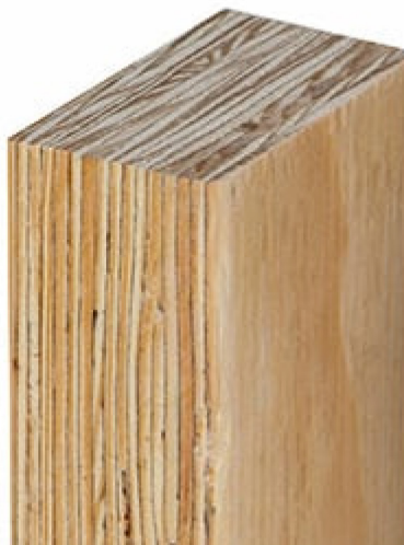
Figure 16 - Lamine veneer lumber. (Photo: Canadian Wood Council 2021)
