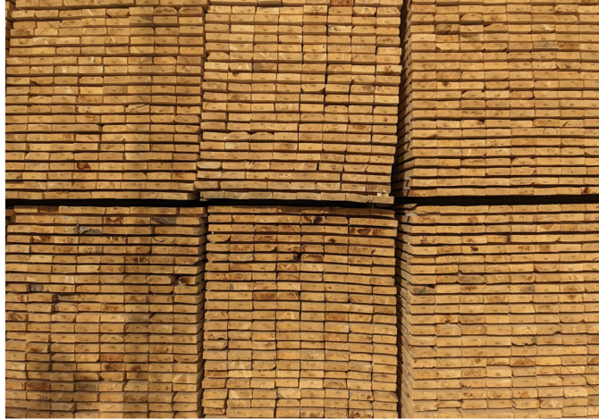
Figure 10 - Softwood lumber stacked and sticker after milling. (Photo: Peter Osborne)
