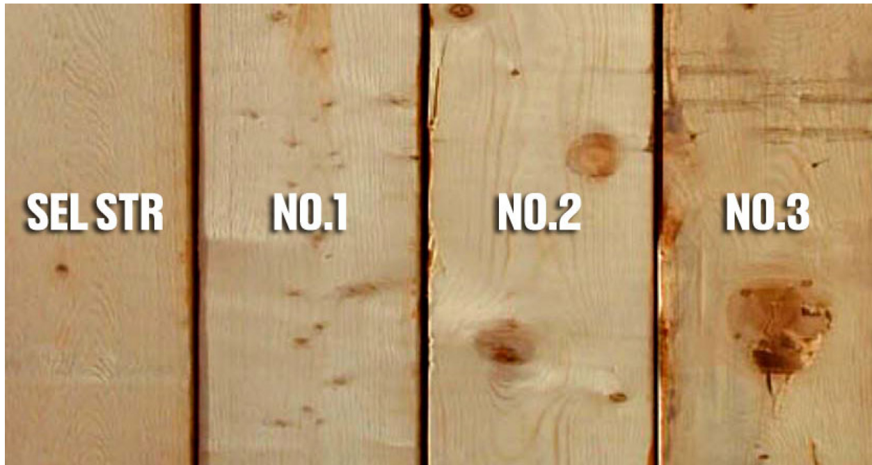
Figure 12 - Visual guide to lumber grades. Visual grading is a method of evaluating lumber by examining its four sides for imperfections that could affect its structural integrity. A trained grader moves quickly along a grading chain to assign each piece of lumber to a visual grade. (Source: "Unraveling the Lumberyard Labyrinth: Your Guide to Lumber Grades," n.d.)
