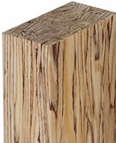
Figure 17 - Parallel strand lumber. (Photo: Canadian Wood Council 2021)
