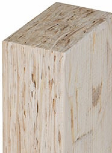
Figure 15 - Laminate strand lumber. (Canadian Wood Council 2021)
