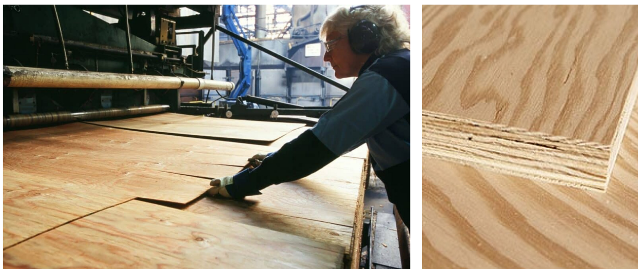
Figure 19 – The plywood manufacturing process. Left: Canadian plywood mill. (Photo: “Naturally:Wood | British Columbia’s Sustainable Forestry Resource,” n.d.). Right: Plywood sheet. (Photo: Canadian Wood Council 2021)
