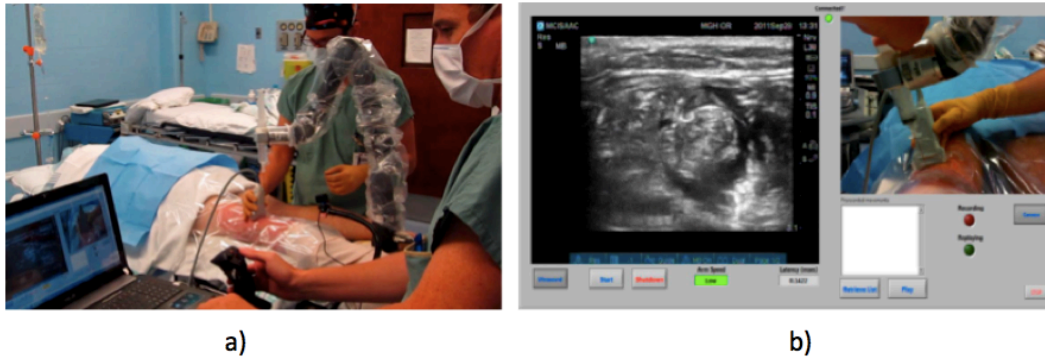
Fig. 35: Views of the Magellan robot assisted ultrasound-guided nerve block (Thomas M Hemmerling et al., 2013). In a) a view of the arm being used on a patient and b) the cockpit view.
