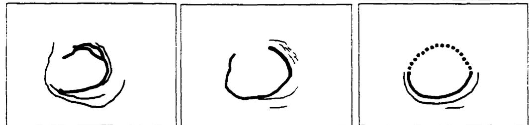
Figure 66. Changing the position and the orientation of the topography has little effect on the final caldera morphology.
