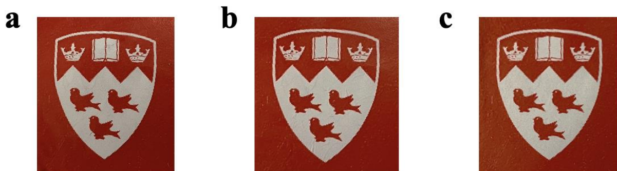
Figure 4.15 The appearance of PVA (a), PVA/CNF (b), and PVA/CNF/PLH (c) films with the background of McGill logo.
