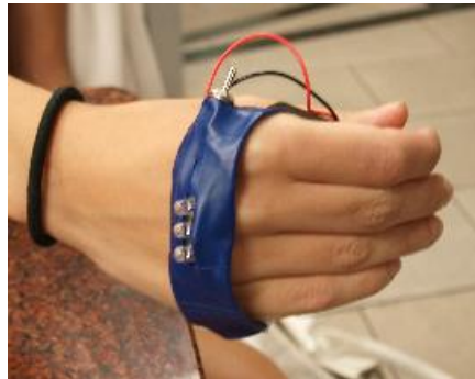
Fig. 3.3: The custom-built sensor strap built for the Videoconferencing Privacy System.
